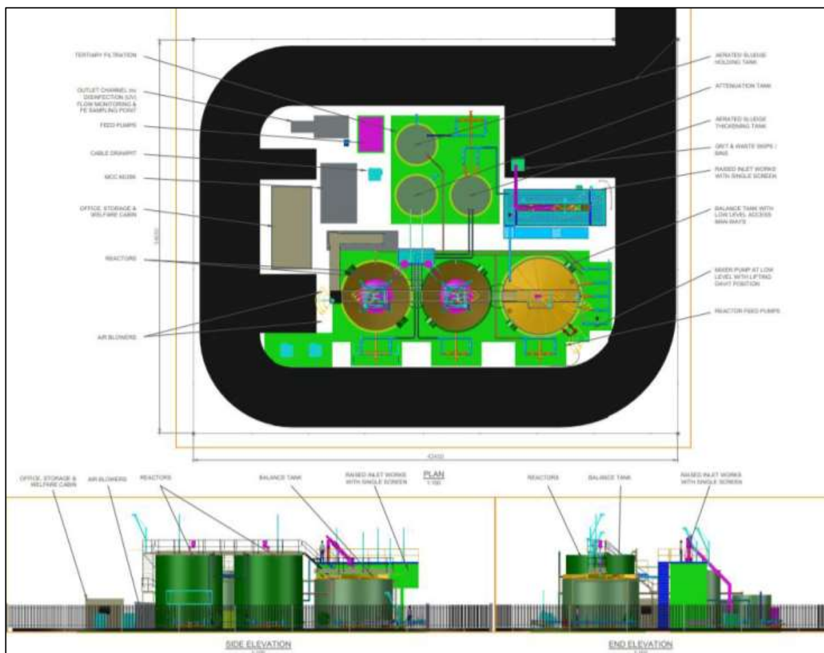
Figure 4.12: Potential Wastewater Treatment Works Layout
