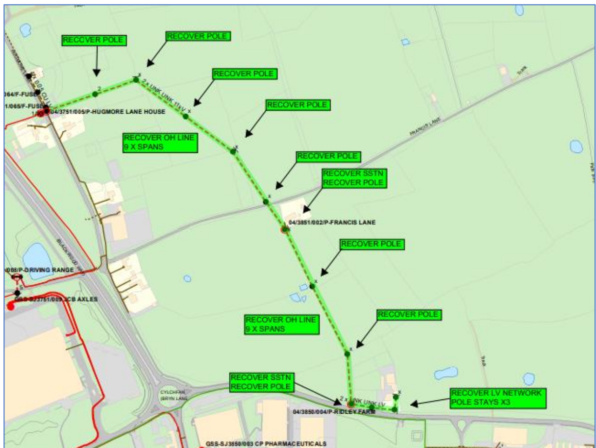
HV overhead Line to be removed
