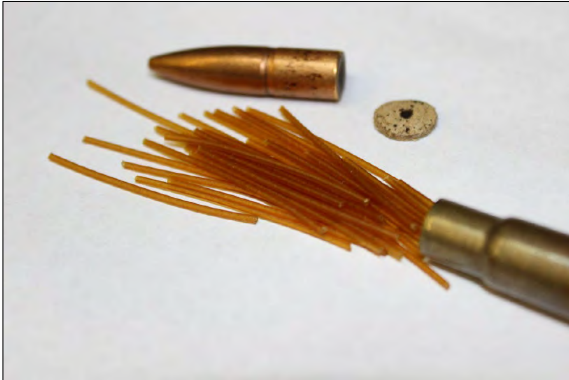
Plate 3 Cordite filaments in a .303 British Rifle cartridge
