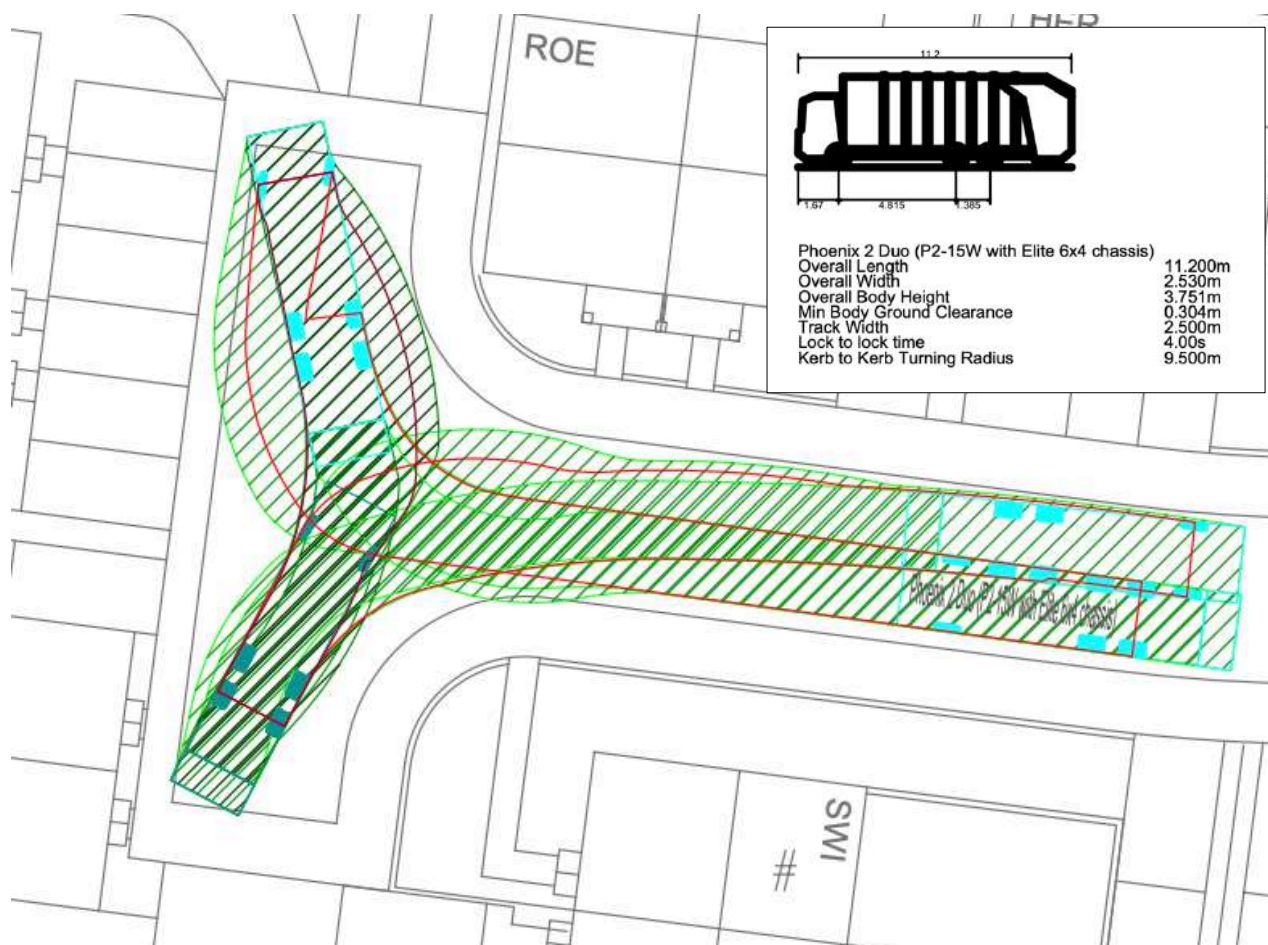
Figure 3.2 : Swept Path Analysis – 11.2m Refuse Collection Vehicle
