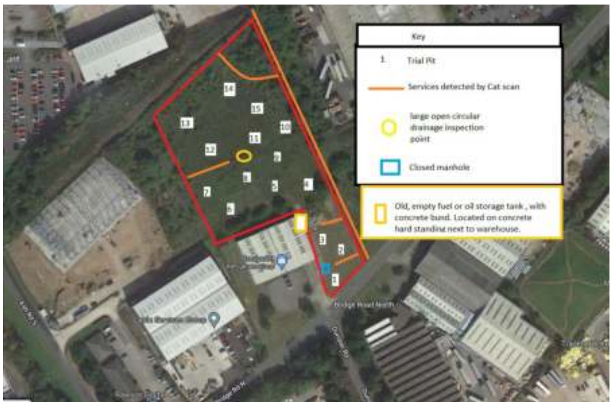
Figure 3: Trial Pit Locations
