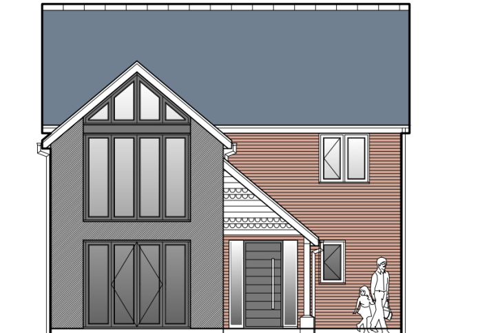
Fig. 4 – Front Elevation of House Type A
