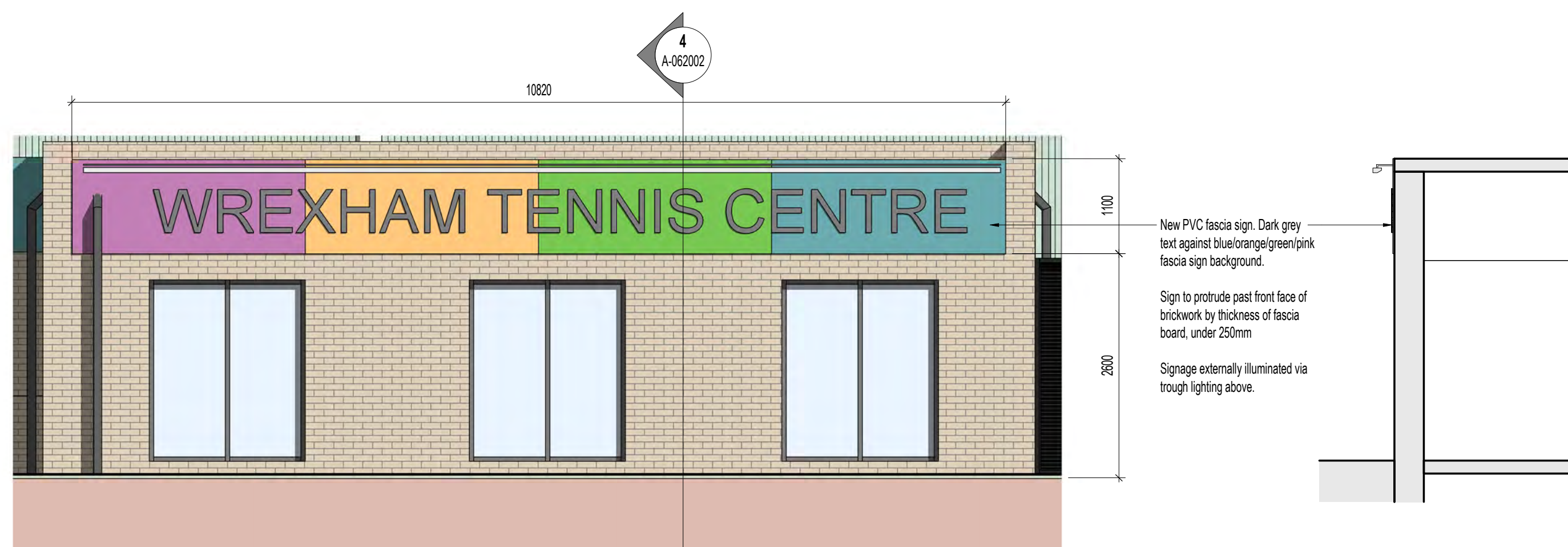
Proposed - West Elevation - Fascia Signage 1 : 50
