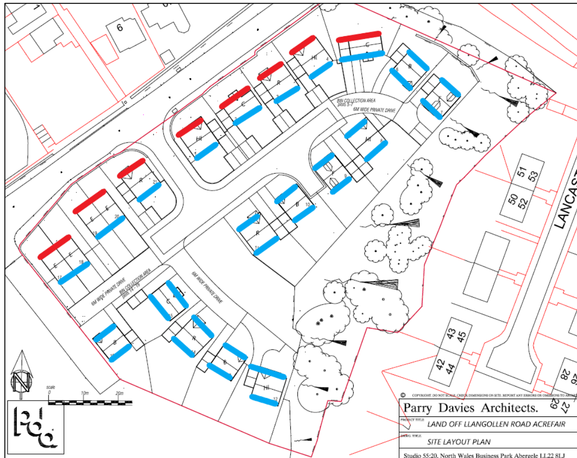
Figure 4.1 - Site layout showing recommended glazing types
