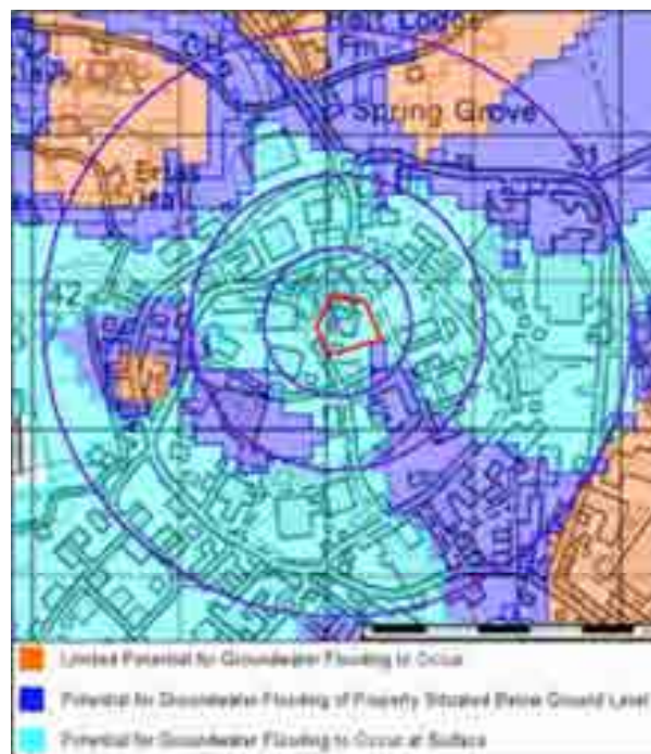
Figure 6: BGS Groundwater Flooding Susceptibility Map (Site location in red)
