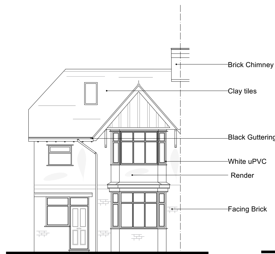
Existing Front Elevation 1:100 View A
