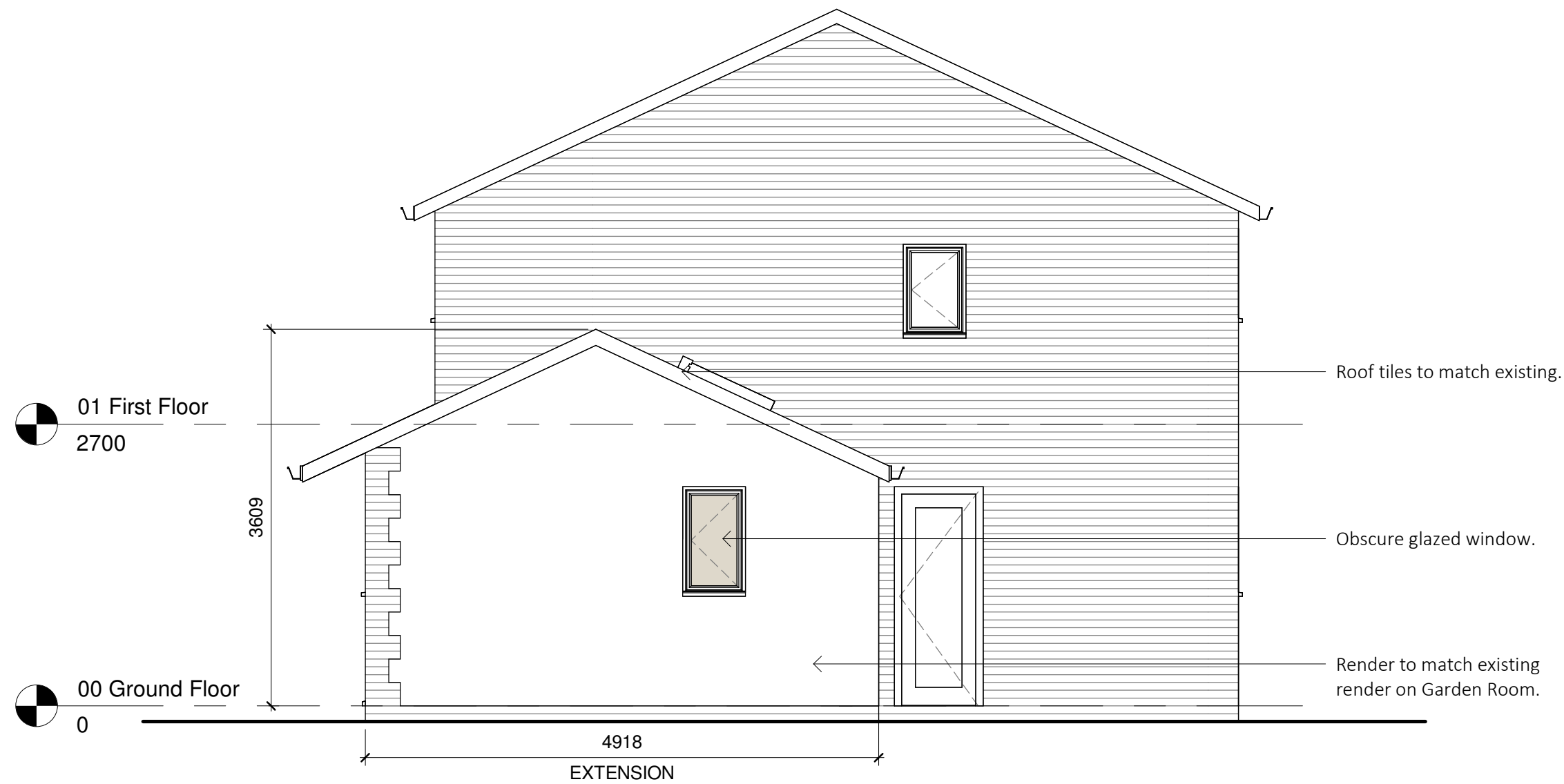
Proposed East Elevation 1 : 50
