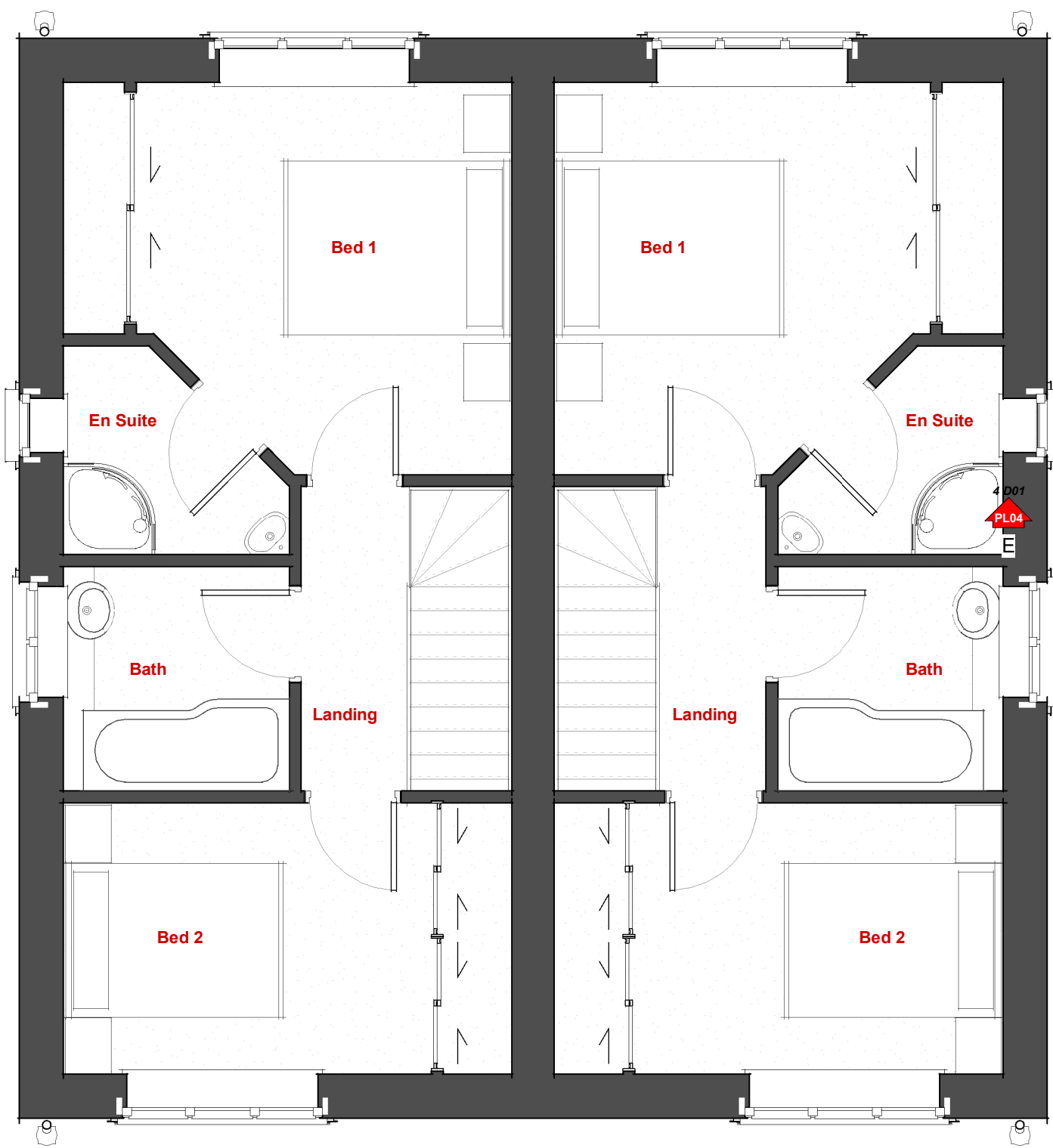
House - First Floor Scale: 1 : 50
