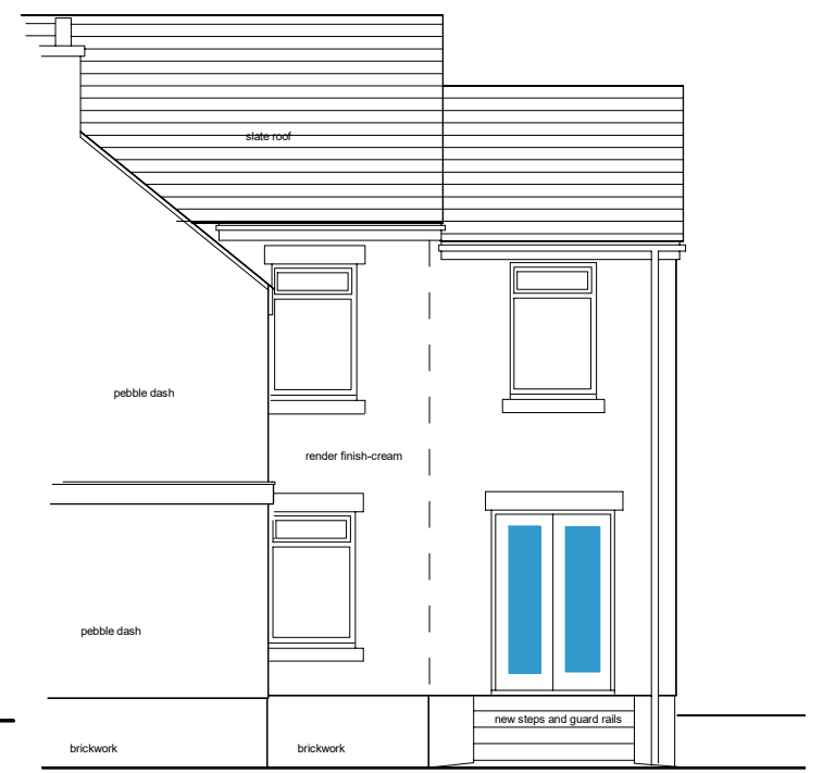
NORTH ELEVATION REAR
