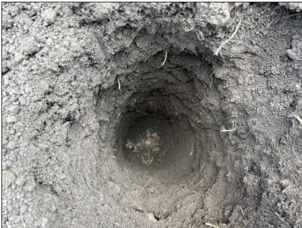
Photograph 9: Photograph shows the nature of the inert cover within the validation hole in the front garden of Plot 349. Photograph taken 26 th April 2022.
