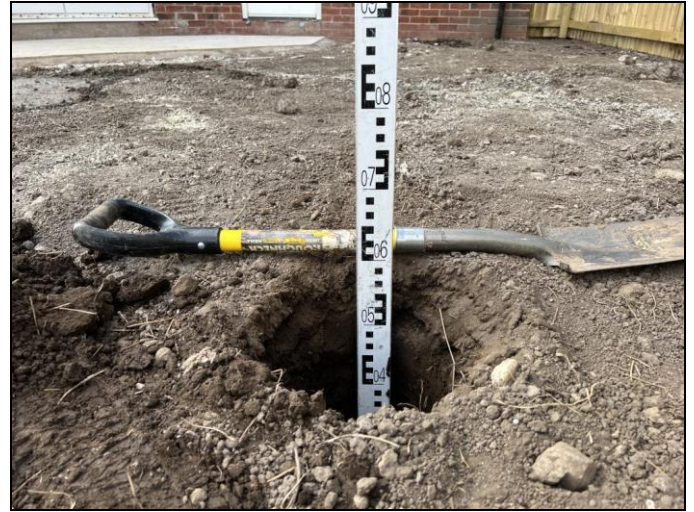
Photographs 4 & 5: Showing the depth of the inert cover and location of the validation hole within the rear garden of Plot 350 and the depth of inert cover achieved. Photographs taken 25 th April 2022.
