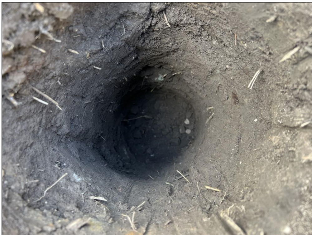
Photograph 6: Photograph shows the nature of the inert cover within the validation hole in the rear garden of Plot 350. Photograph taken 25 th April 2022.
