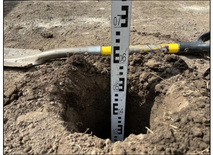
Photographs 1 & 2: Showing the depth of the inert cover and location of the validation hole within the rear garden of Plot 349 and the depth of inert cover achieved. Photographs taken 25 th April 2022.
