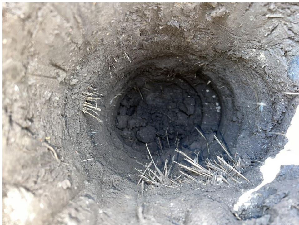
Photograph 3: Photograph shows the nature of the inert cover within the validation hole in the rear garden of Plot 349. Photograph taken 25 th April 2022.
