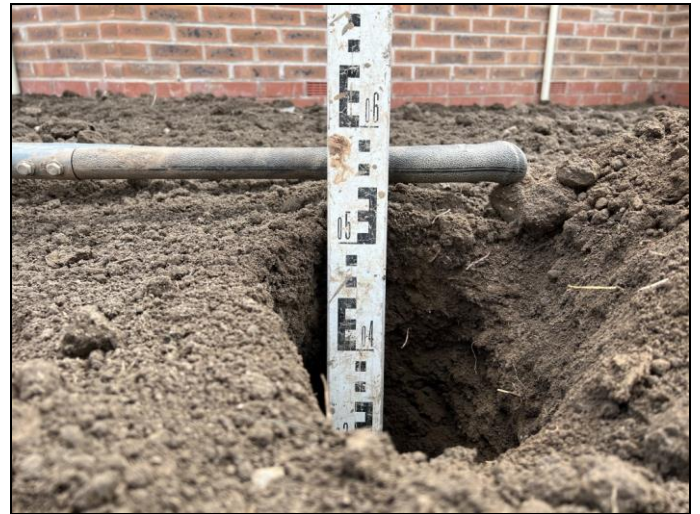
Photographs 7 & 8: Showing the depth of the inert cover and location of the validation hole within the front garden of Plot 349 and the depth of inert cover achieved. Photographs taken 26 th April 2022.
