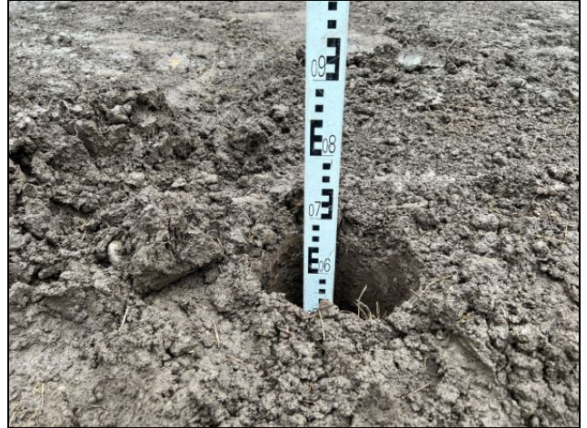
Photographs 1 & 2: Showing the depth of the inert cover and location of the validation hole within the rear garden of Plot 348 and the depth of inert cover achieved. Photographs taken 3 rd March 2022.
