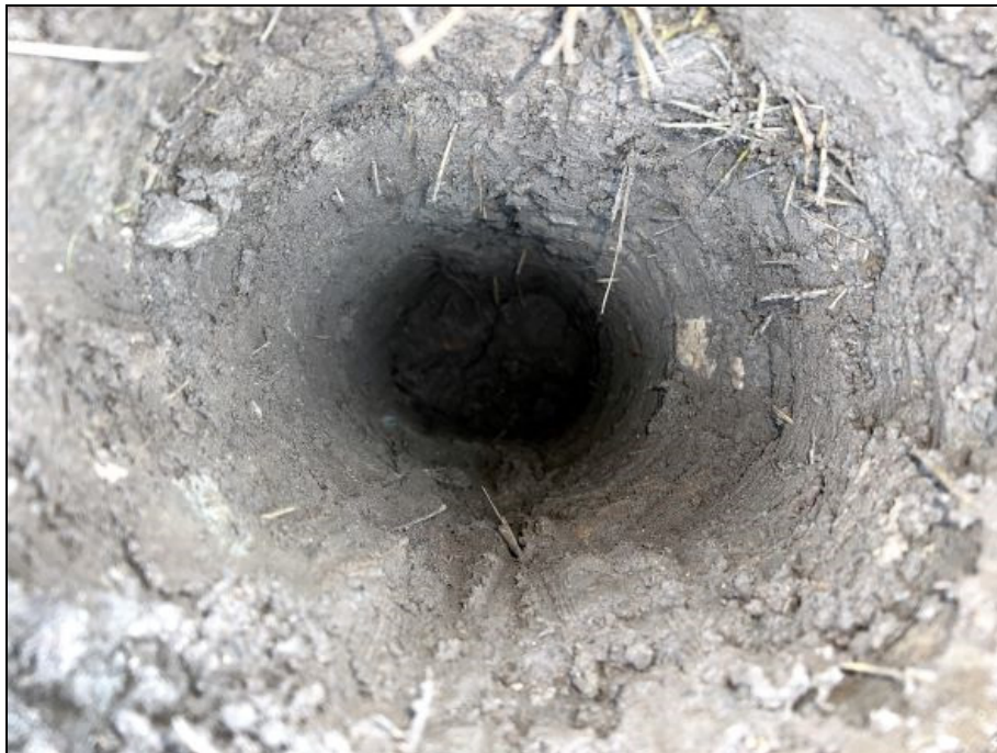
Photograph 3: Photograph shows the nature of the inert cover within the validation hole in the rear garden of Plot 348. Photograph taken 3 rd March 2022.
