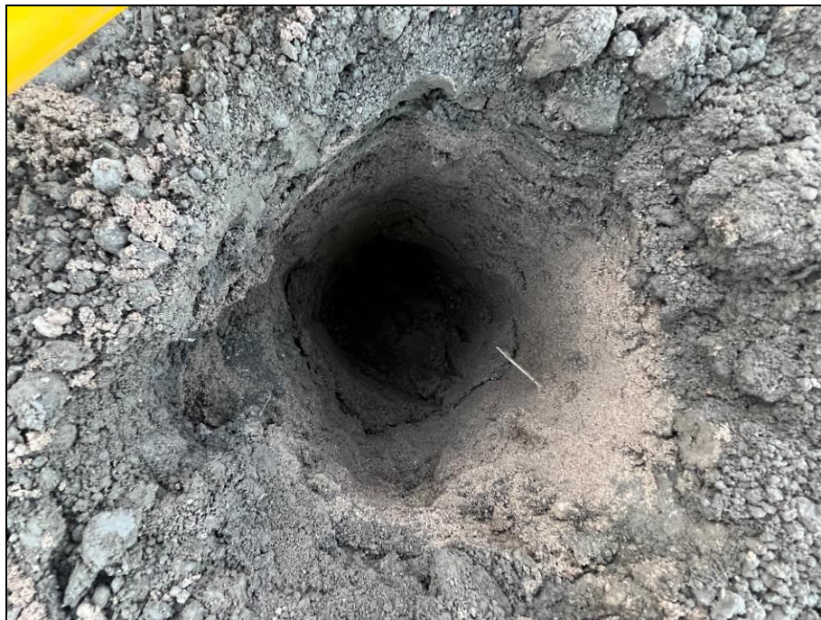
Photograph 15: Shows the composition of the inert cover within the validation hole in the rear garden of Plot 250. Photograph taken 24 th November 2023.
