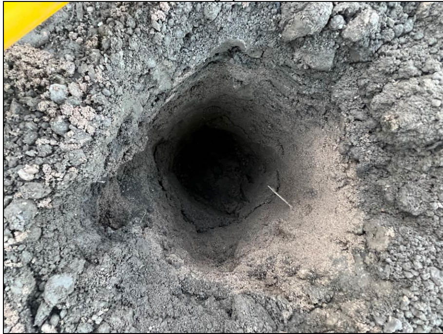
Photograph 12: Shows the composition of the inert cover within the validation hole in the rear garden of Plot 249. Photograph taken 23 rd November 2023.
