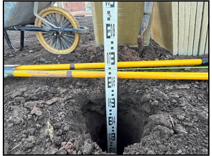
Photographs 13 & 14: Showing the location of the validation hole within the rear garden of Plot 250 and the depth of inert cover achieved. Photographs taken 24 th November 2023.
