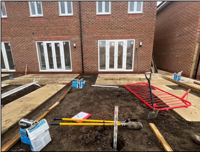
Photographs 7 & 8: Showing the location of the validation hole within the rear garden of Plot 248 and the depth of inert cover achieved. Photographs taken 24 th November 2023.
