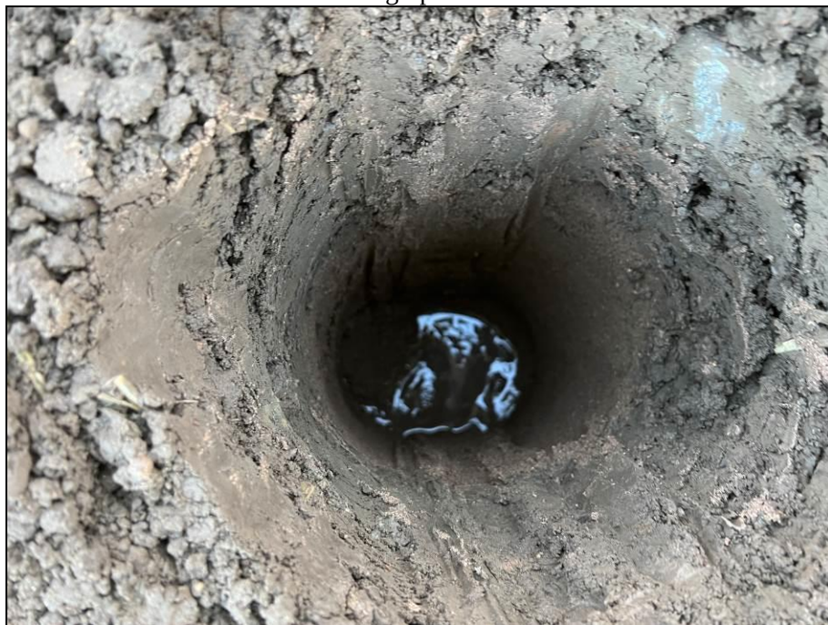
Photograph 3: Shows the composition of the inert cover within the validation hole in the rear garden of Plot 246. Photograph taken 23 rd November 2023.
