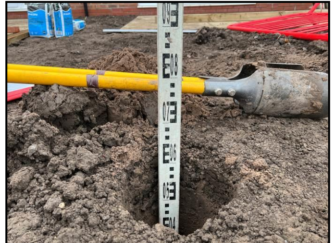
Photographs 7 & 8: Showing the location of the validation hole within the rear garden of Plot 248 and the depth of inert cover achieved. Photographs taken 24 th November 2023.
