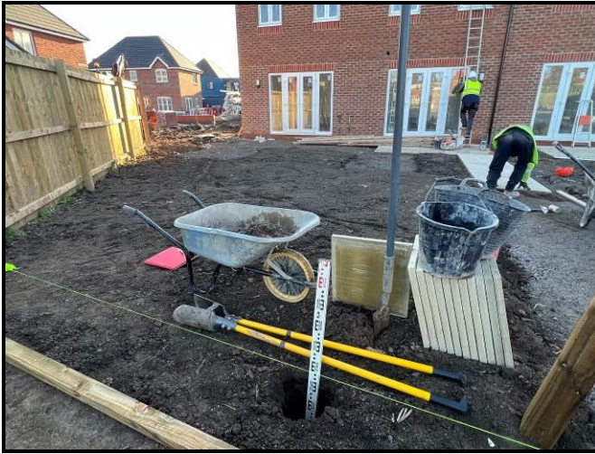
Photographs 10 & 11: Showing the location of the validation hole within the rear garden of Plot 249 and the depth of inert cover achieved. Photographs taken 23 rd November 2023.
