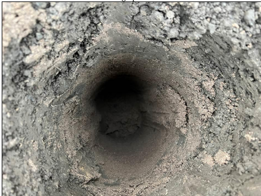
Photograph 9: Shows the composition of the inert cover within the validation hole in the rear garden of Plot 248. Photograph taken 24 th November 2023.
