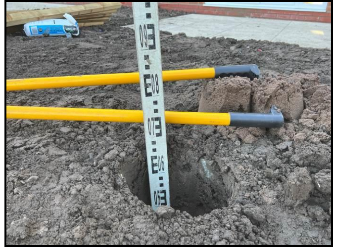
Photographs 1 & 2: Showing the location of the validation hole within the rear garden of Plot 246 and the depth of inert cover achieved. Photographs taken 23 rd November 2023.
