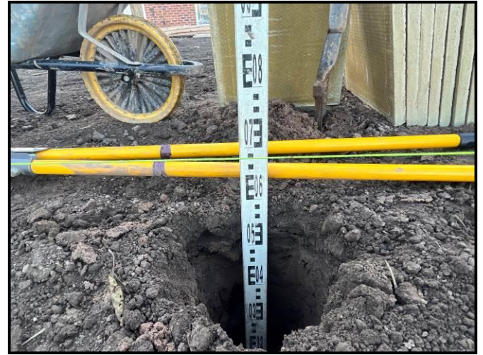
Photographs 10 & 11: Showing the location of the validation hole within the rear garden of Plot 249 and the depth of inert cover achieved. Photographs taken 23 rd November 2023.
