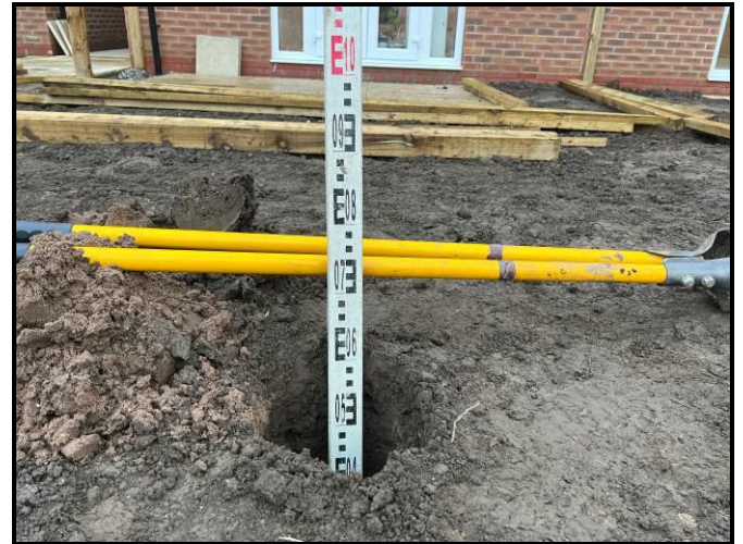
Photographs 4 & 5: Showing the location of the validation hole within the rear garden of Plot 247 and the depth of inert cover achieved. Photographs taken 24 th November 2023.
