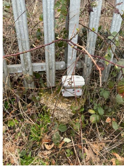
Figure 2 – vibration monitor at site boundary
