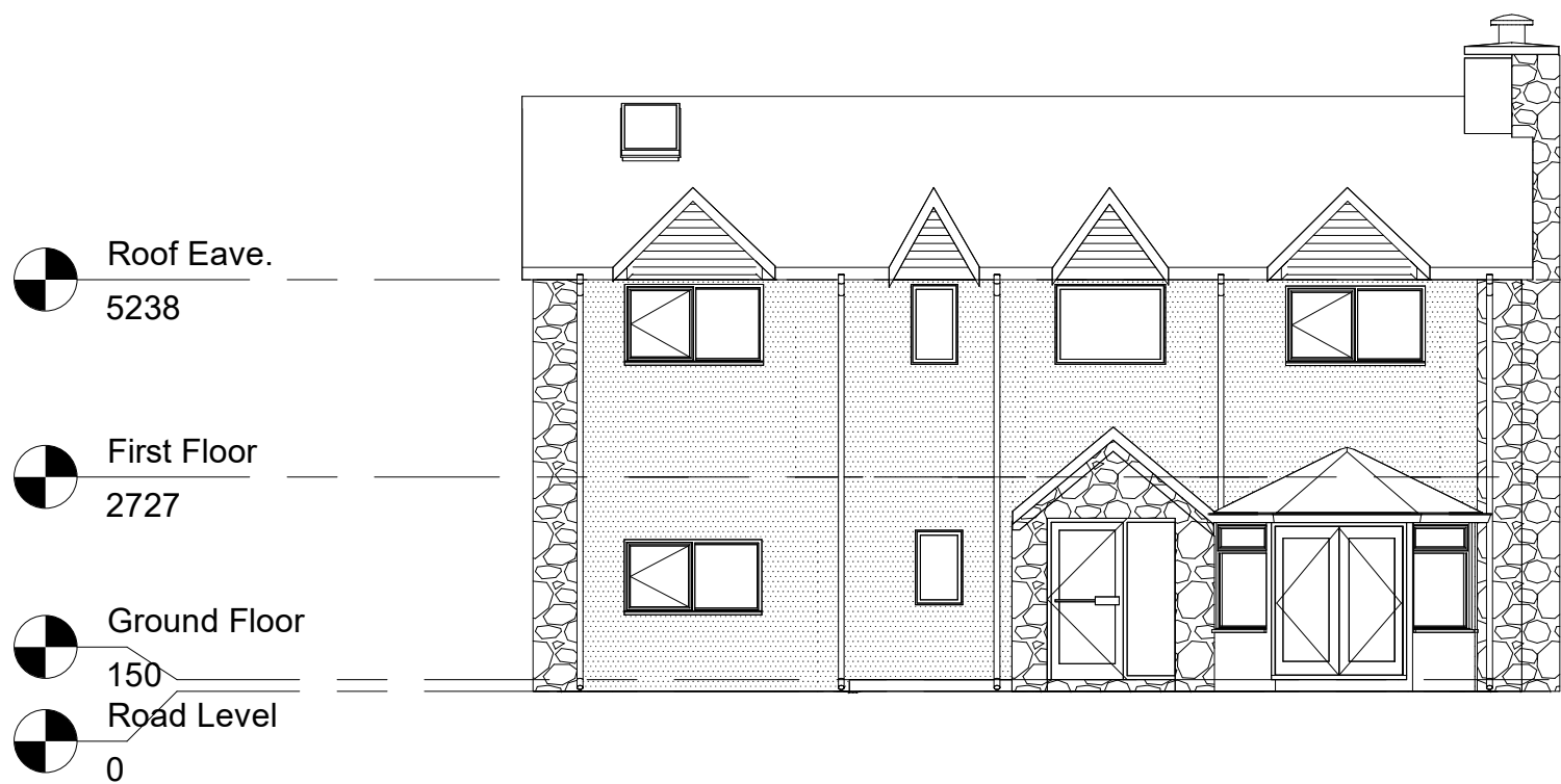
Existing Front Elevation 1 : 100
