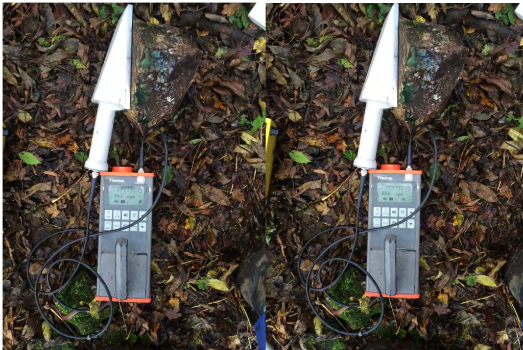
Figure A10 [REDACTED] beta and alpha count rates from naturally occurring radioactivity in a ceramic glazed brick.
