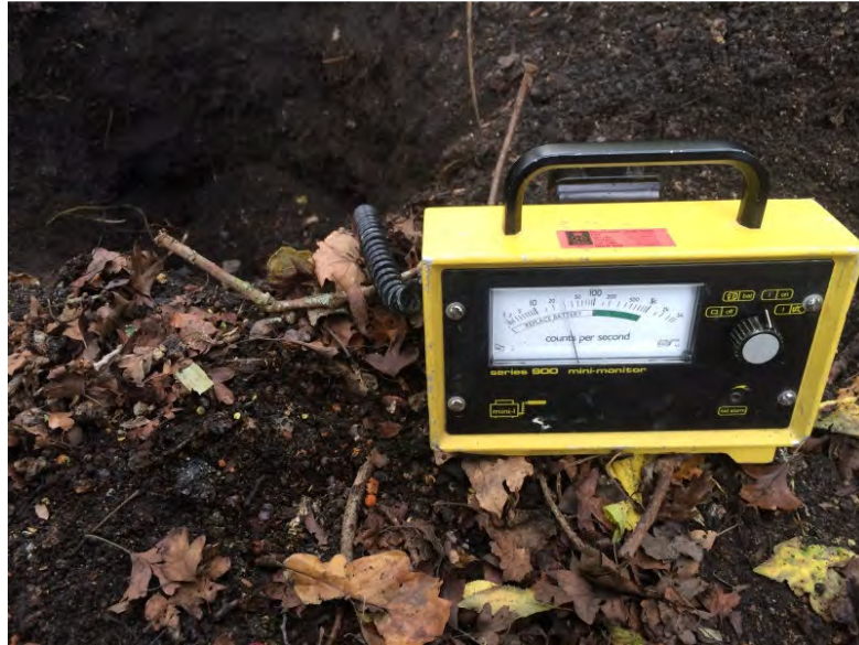
Figure A9 [REDACTED] count rates due to naturally occurring radioactivity in ash.
