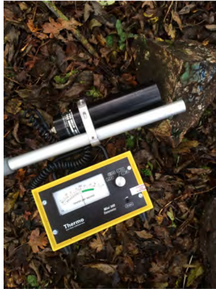
Figure A11 [REDACTED] gamma count rates from naturally occurring radioactivity in a ceramic glazed brick.
