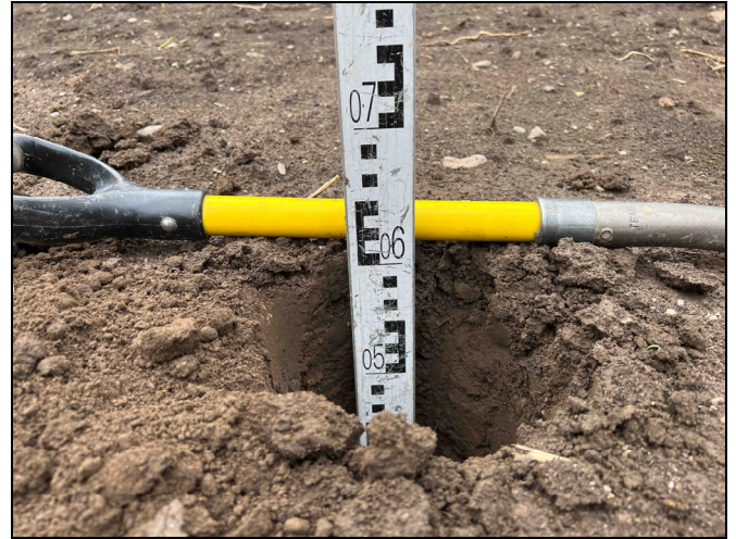
Photographs 4 & 5: Showing the depth of the inert cover and location of the validation hole within the rear garden of Plot 351 and the depth of inert cover achieved. Photographs taken 20 th June 2023.
