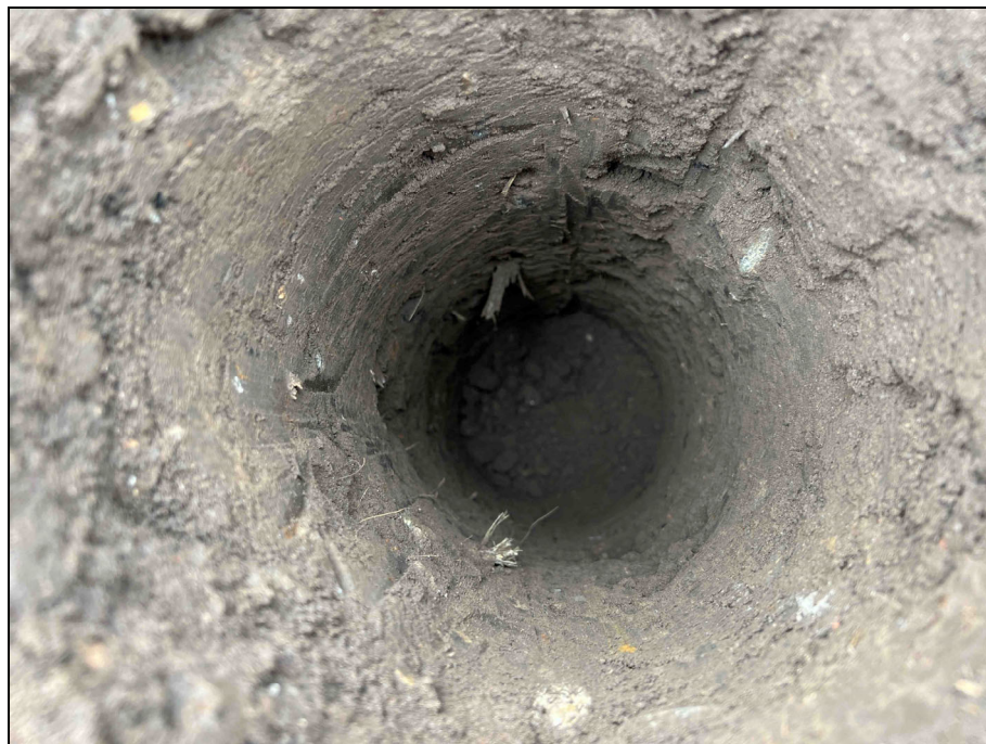
Photograph 6: Photograph shows the nature of the inert cover within the validation hole in the rear garden of Plot 351. Photograph taken 20 th June 2023.
