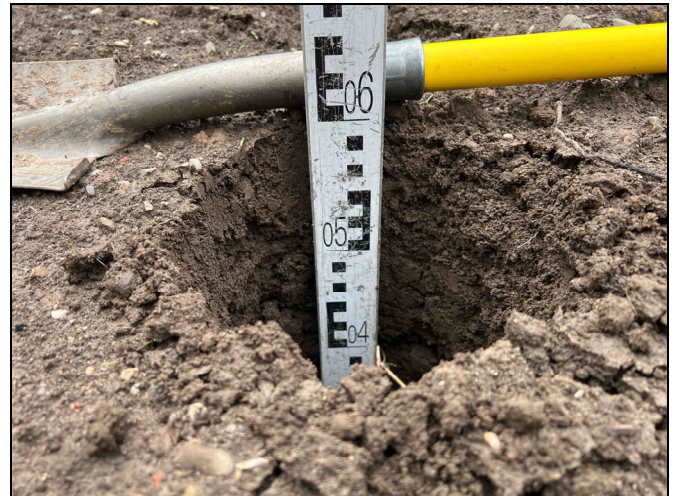
Photographs 7 & 8: Showing the depth of the inert cover and location of the validation hole within the rear garden of Plot 352 and the depth of inert cover achieved. Photographs taken 20 th June 2023.
