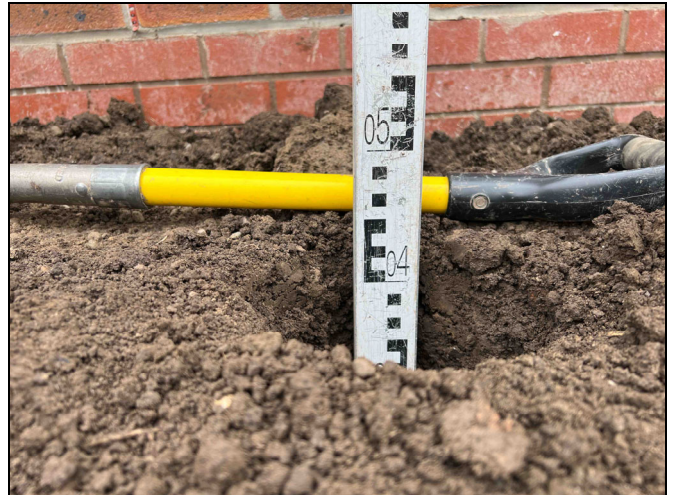
Photographs 1 & 2: Showing the depth of the inert cover and location of the validation hole within the front garden of Plot 351 and the depth of inert cover achieved. Photographs taken 20 th June 2023.
