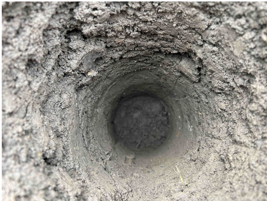
Photograph 9: Photograph shows the nature of the inert cover within the validation hole in the front garden of Plot 352. Photograph taken 20 th June 2023.
