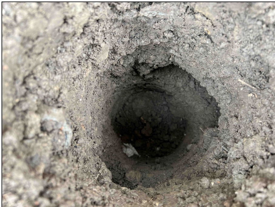
Photograph 3: Photograph shows the nature of the inert cover within the validation hole in the front garden of Plot 351. Photograph taken 20 th June 2023.
