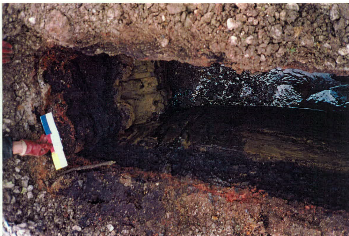
PLATE 25: Trial Pit TP 20. Fill material overlying sand. Coal tar like material can be seen seeping into the pit. This is located in the vicinity of the former CWG Plant.
