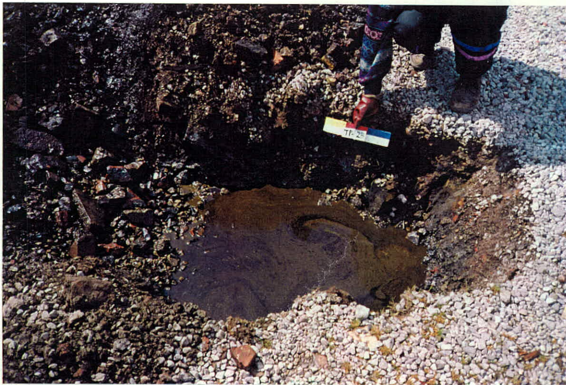
PLATE 28: Trial Pit TP 23. Showing the fill material within the Tar Well. Water sample location TP 23.
