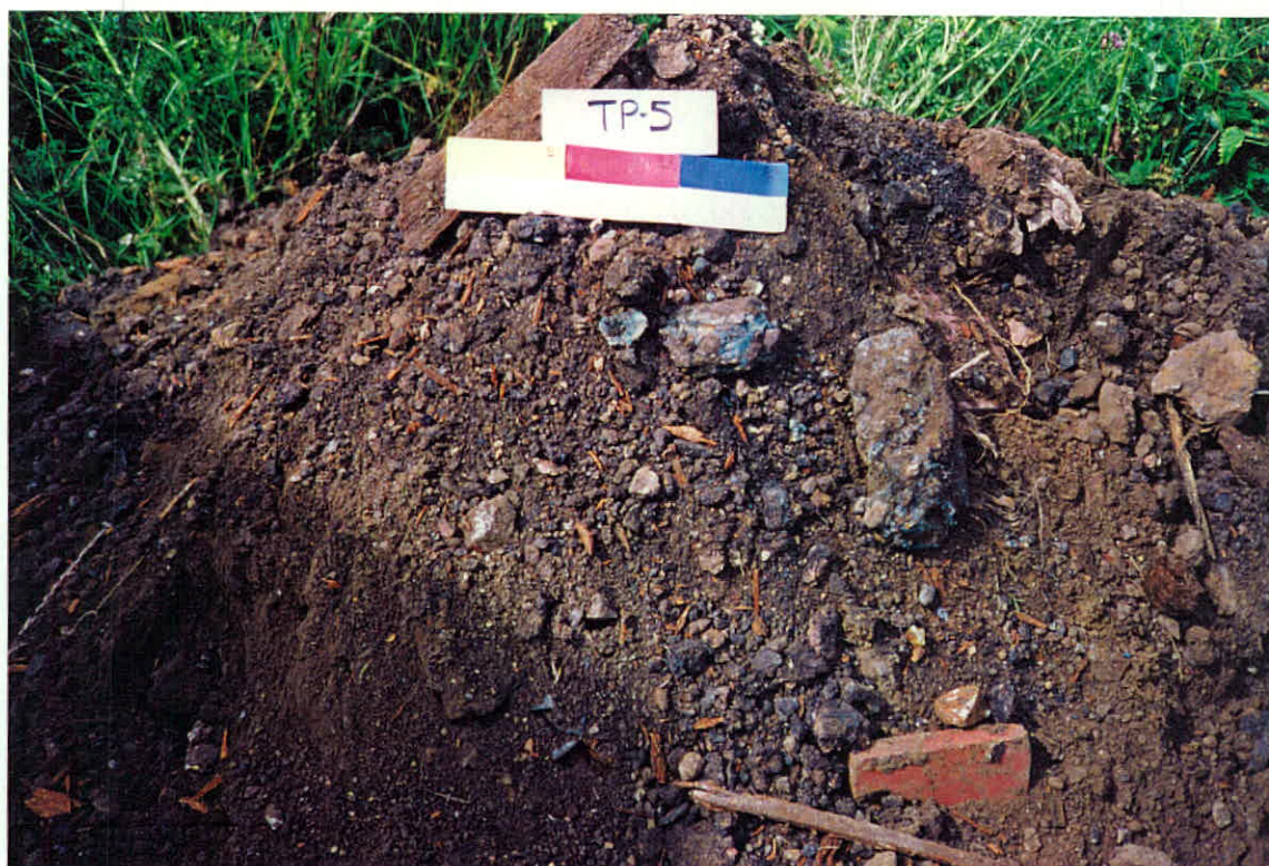
PLATE 20: Spent oxide [REDACTED] from Trial Pit TP 5.
