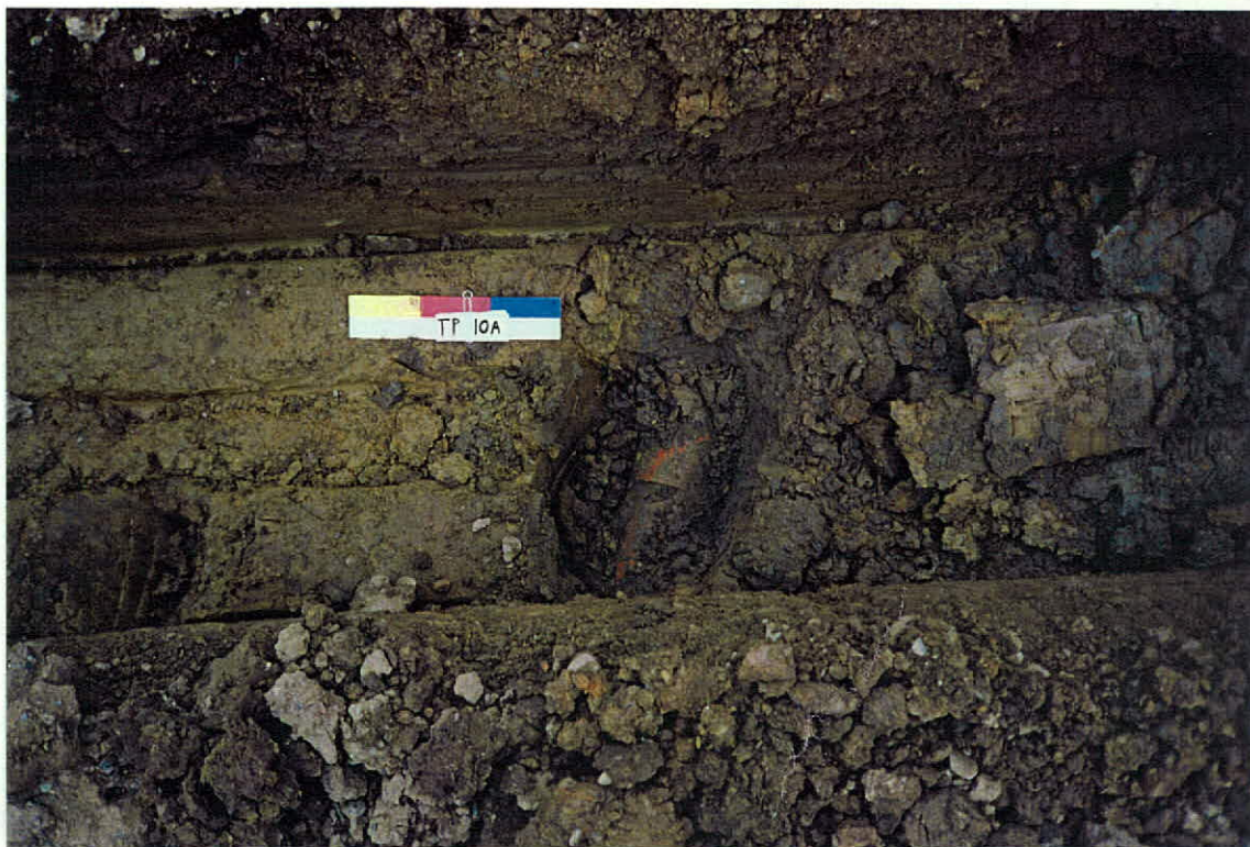
PLATE 22: Trial Pit 10A in the vicinity of the former Oil-Gas Plant, showing the clay drift deposit.
