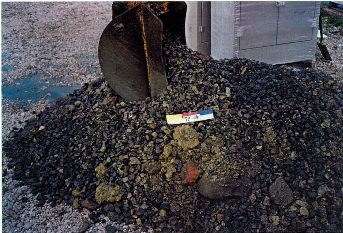
PLATE 30: Trial Pit TP24. Showing the fill material within the former Effluent Well.
