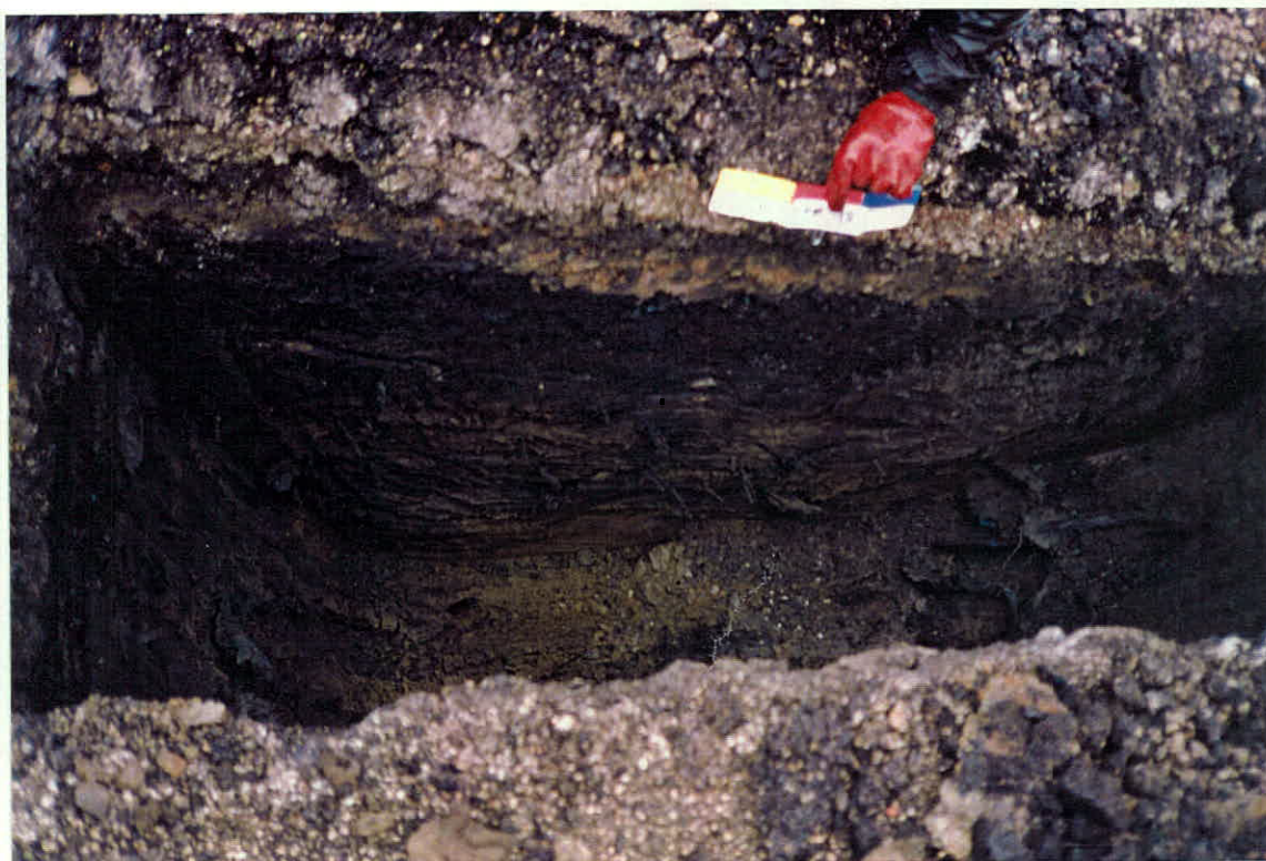
PLATE 24: Trial Pit 18 showing fill material containing tree roots.
