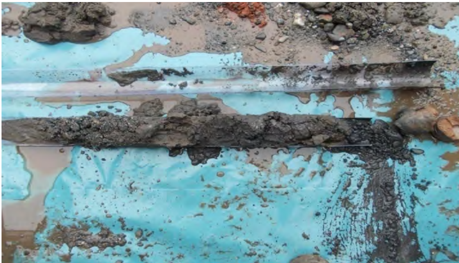
Plate 8: BH2 - Training Centre – Window sample (approx 1m sample liner length 26-11-13)
