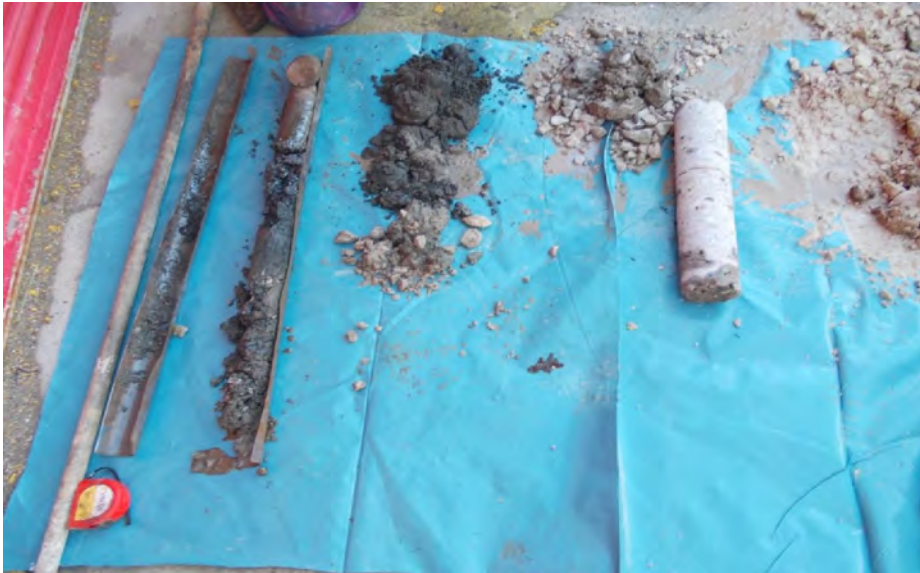
Plate 9: BH23 Garage – Window sample (approx 1m sample liner lengths 09-12-2013)
