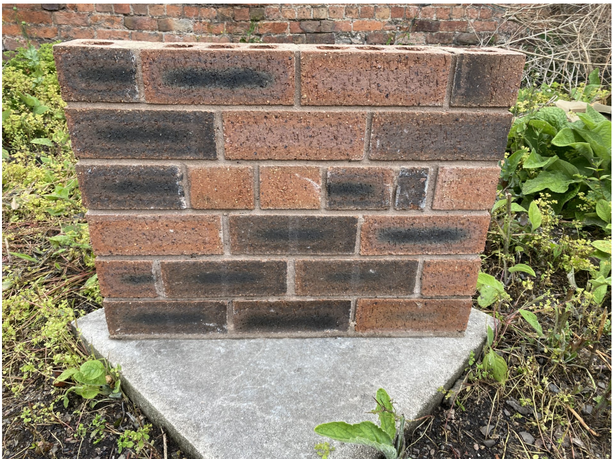
Sample mortar mix for wall with approved Snowie Heritage 73mm Dragwire brick . Mortar mix = 1 part Hanson NHL 3.5 hydraulic Lime 3 parts coarse sand from Borrás quarry.
