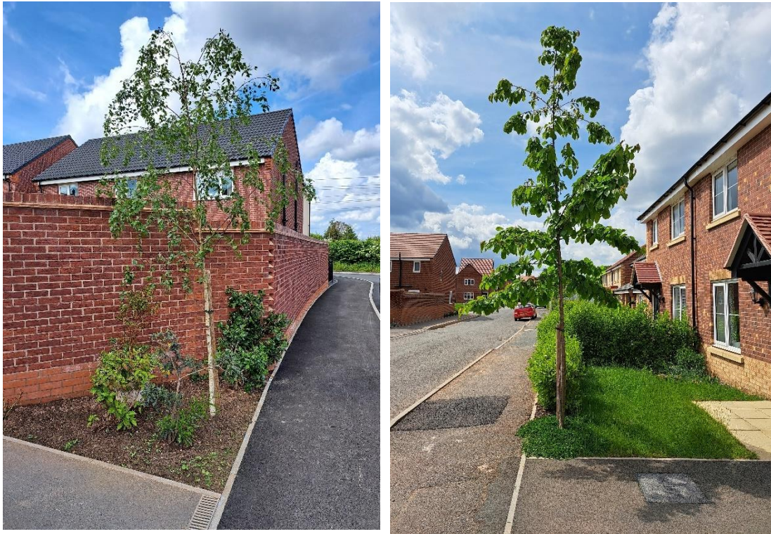
Figure 3 Poor planting practices to avoid: Restricted rooting volumes, impermeable surfacing and planting trees near underground services/drainage runs
