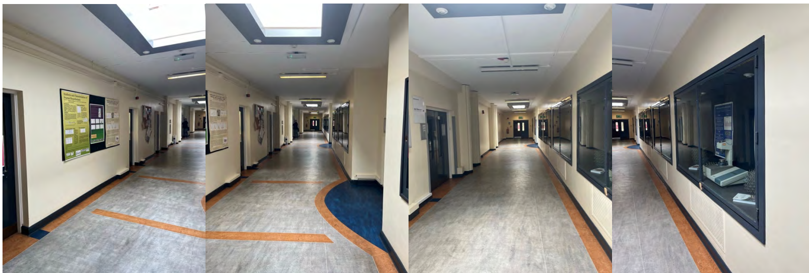
Fig 9. Corridor C showcase cupboards, which are to be adapted to allow viewing from the corridor into the lab and vice versa. A new glass window will be inserted into the corridor wall between the corridor and Room C43. Please refer to the proposed plan on page 27 and Proposed elevation B-B on Page 28.
