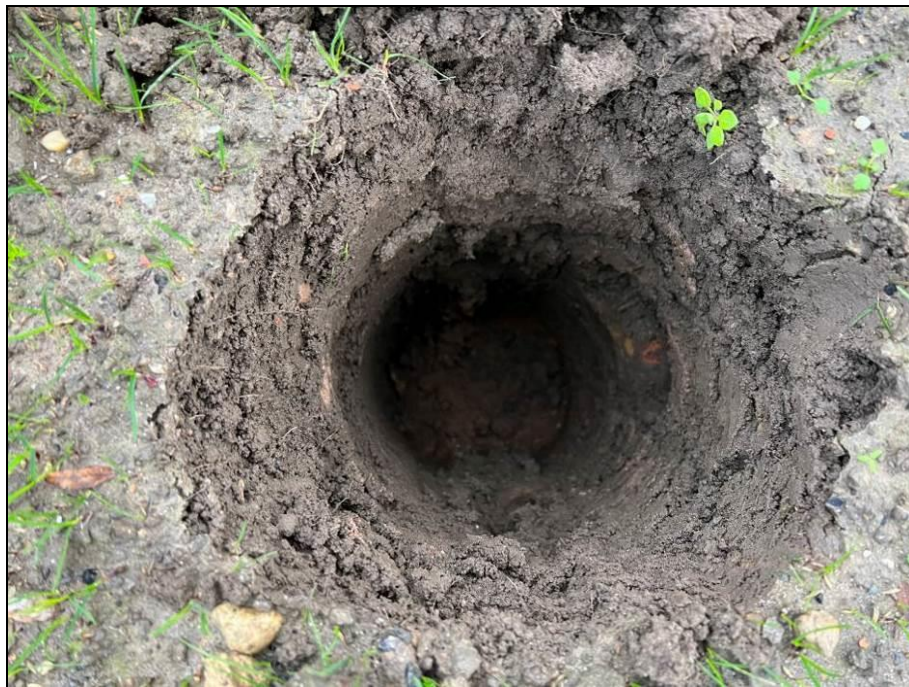
Photograph 15: Shows the composition of the inert cover within the validation hole in the POS Area. Photograph taken 24 th November 2023.
