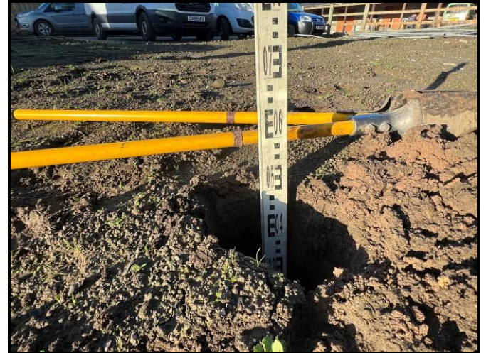
Photographs 1 & 2: Showing the location of the validation hole within the POS Area and the depth of inert cover achieved. Photographs taken 23 rd November 2023.
