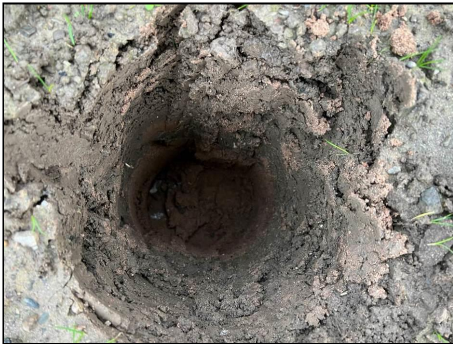
Photograph 12: Shows the composition of the inert cover within the validation hole in the POS Area. Photograph taken 24 th November 2023.
