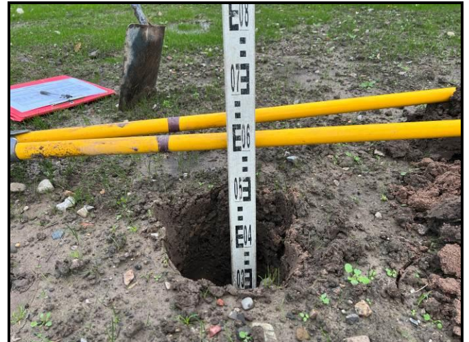
Photographs 10 & 11: Showing the location of the validation hole within the POS Area and the depth of inert cover achieved. Photographs taken 24 th November 2023.
