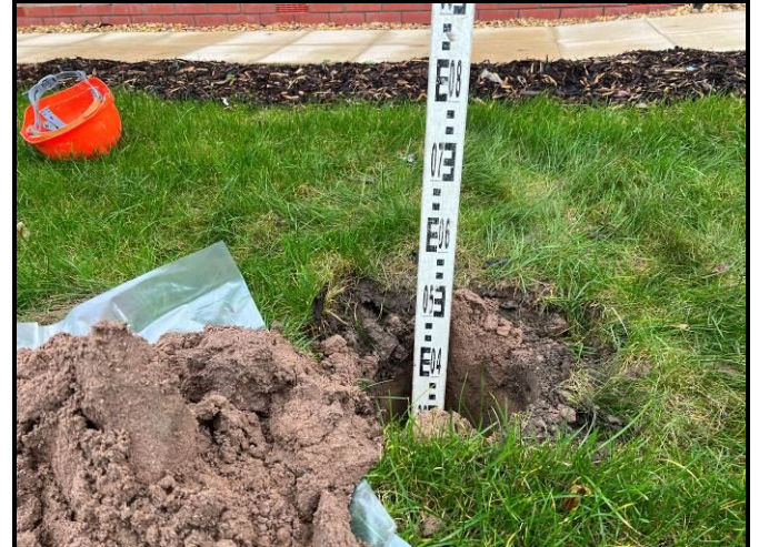
Photographs 7 & 8: Showing the location of the validation hole within the POS Area and the depth of inert cover achieved. Photographs taken 24 th November 2023.
