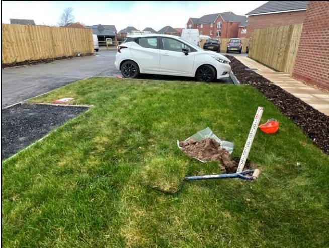
Photographs 7 & 8: Showing the location of the validation hole within the POS Area and the depth of inert cover achieved. Photographs taken 24 th November 2023.
