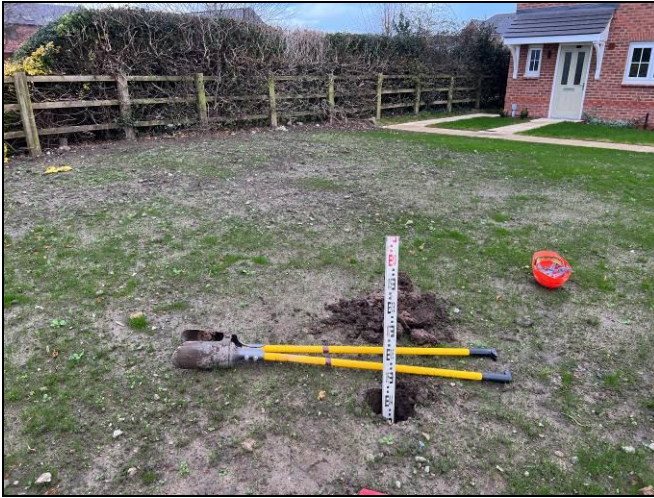
Photographs 13 & 14: Showing the location of the validation hole within the POS Area and the depth of inert cover achieved. Photographs taken 24 th November 2023.
