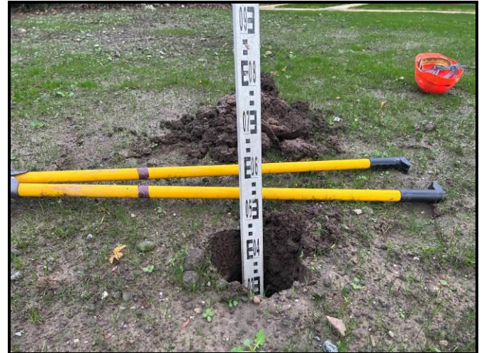
Photographs 13 & 14: Showing the location of the validation hole within the POS Area and the depth of inert cover achieved. Photographs taken 24 th November 2023.
