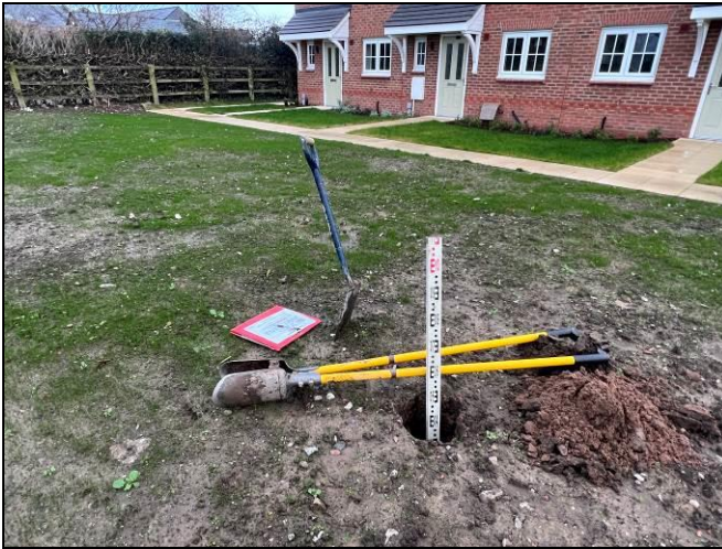
Photographs 10 & 11: Showing the location of the validation hole within the POS Area and the depth of inert cover achieved. Photographs taken 24 th November 2023.
