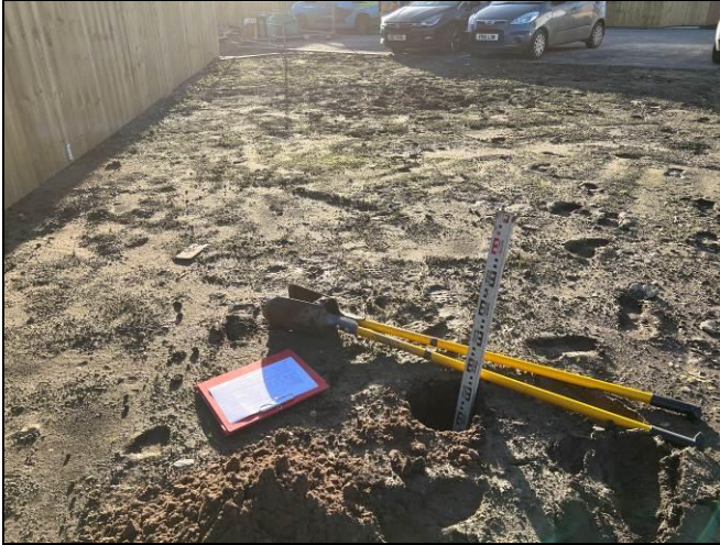
Photographs 4 & 5: Showing the location of the validation hole within the POS Area and the depth of inert cover achieved. Photographs taken 23 rd November 2023.
