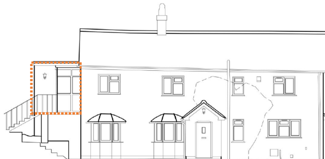
Modern extension demolished down to first floor slab for new roof terrace. (Areas of change highlighted in orange)
