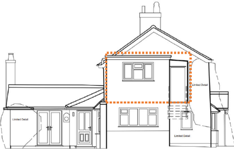
Extension demolished down to first floor slab for new roof terrace.
