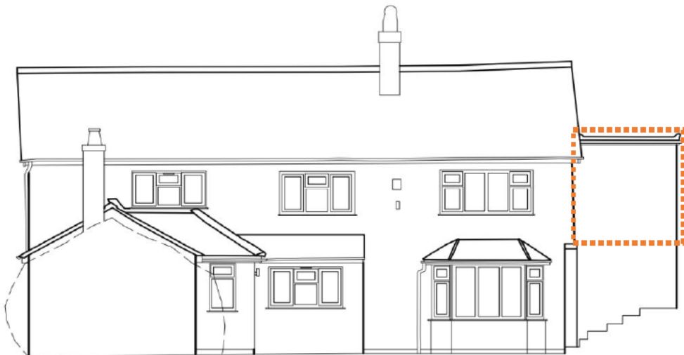
Modern extension demolished down to first floor slab for new roof terrace. (Areas of change highlighted in orange)
