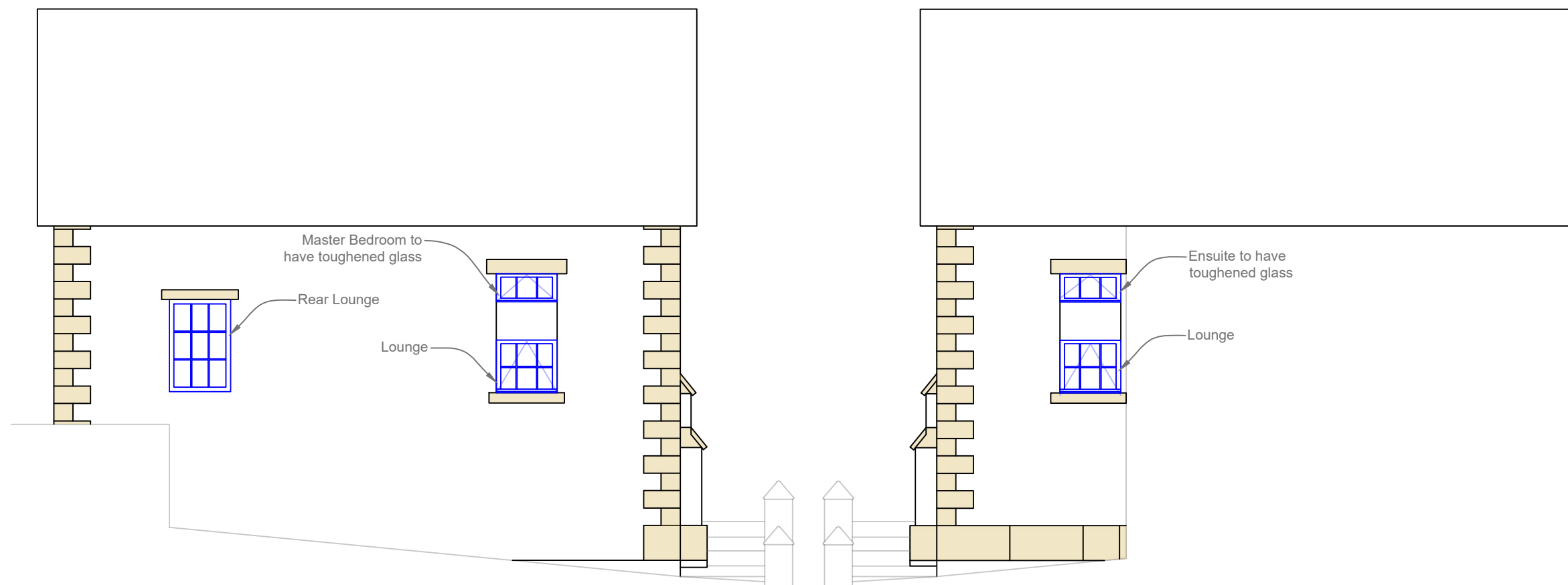
Side Elevation West Facing - 3 units to replace
