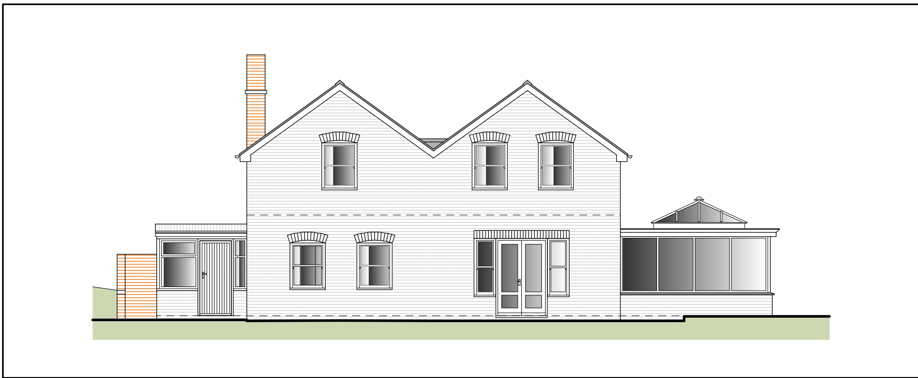
3 EXISTING FRONT ELEVATION 1 : 100
