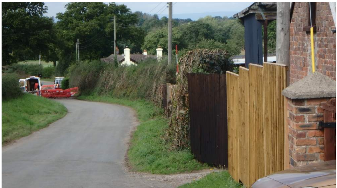
PHOTOGRAPH 10 Visibility from 60m in a easterly direction looking towards the access The photograph is zoomed in towards the access and shows a red & white ranging pole marking 2.4m
