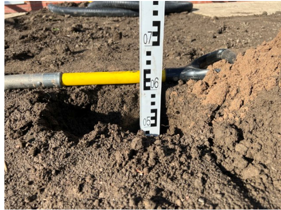
Photographs 1 & 2: Showing the depth of the inert cover and location of the validation hole within the rear garden of Plot 231 and the depth of inert cover achieved. Photographs taken 13 th September 2023.
