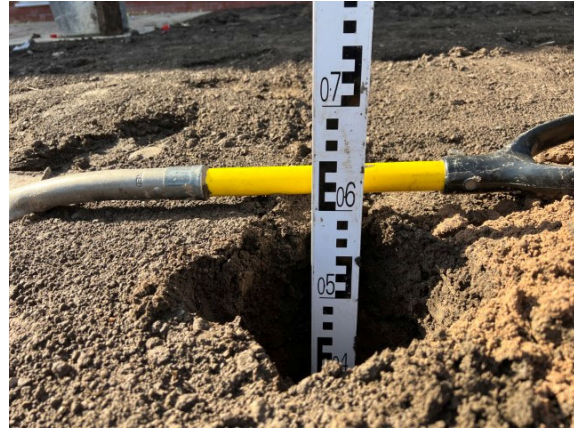
Photographs 16 & 17: Showing the depth of the inert cover and location of the validation hole within the rear garden of Plot 236 and the depth of inert cover achieved. Photographs taken 13 th September 2023.
