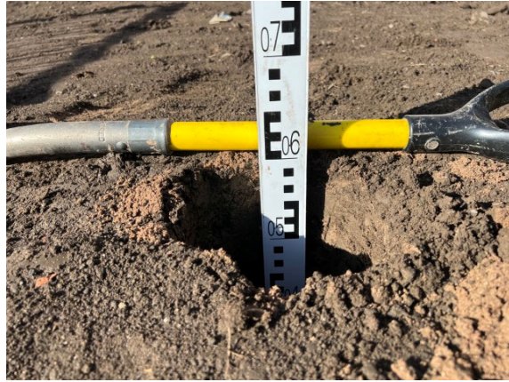
Photographs 4 & 5: Showing the depth of the inert cover and location of the validation hole within the rear garden of Plot 232 and the depth of inert cover achieved. Photographs taken 13 th September 2023.
