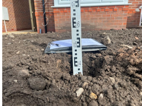
Photographs 22 & 23: Showing the depth of the inert cover and location of the validation hole within the front garden of Plot 234 and the depth of inert cover achieved. Photographs taken 20 th September 2023.
