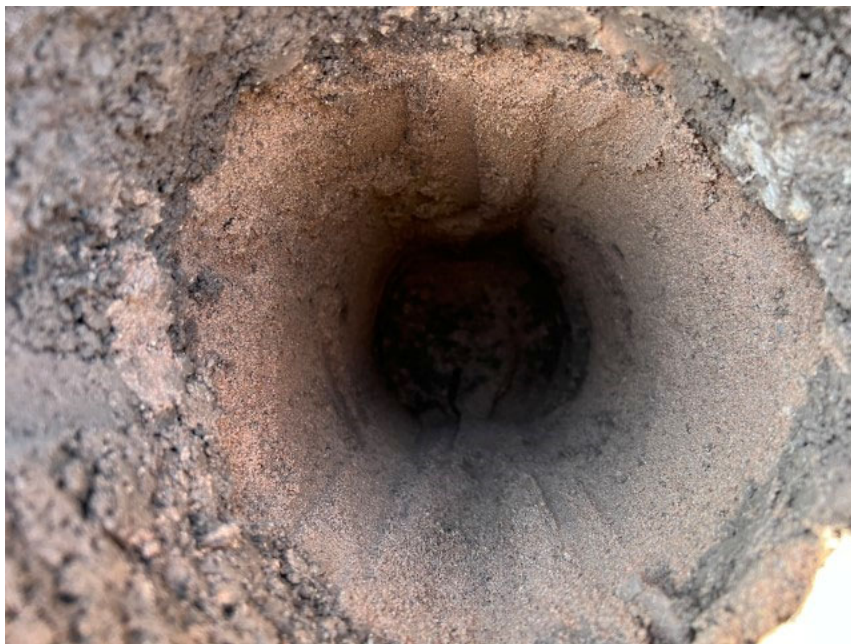
Photograph 18: Photograph shows the nature of the inert cover within the validation hole in the rear garden of Plot 236. Photograph taken 13 th September 2023.
