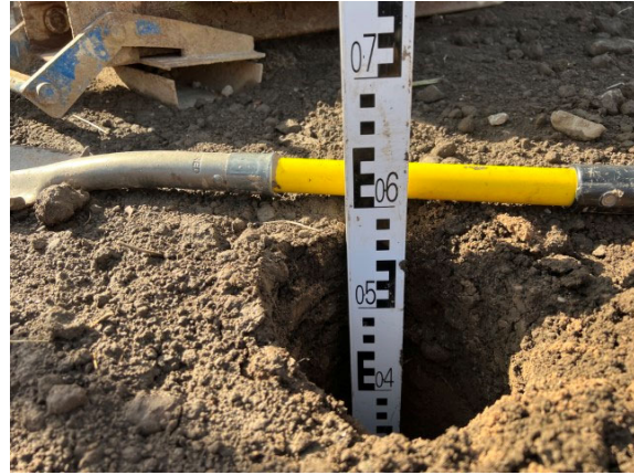
Photographs 19 & 20: Showing the depth of the inert cover and location of the validation hole within the rear garden of Plot 237 and the depth of inert cover achieved. Photographs taken 13 th September 2023.
