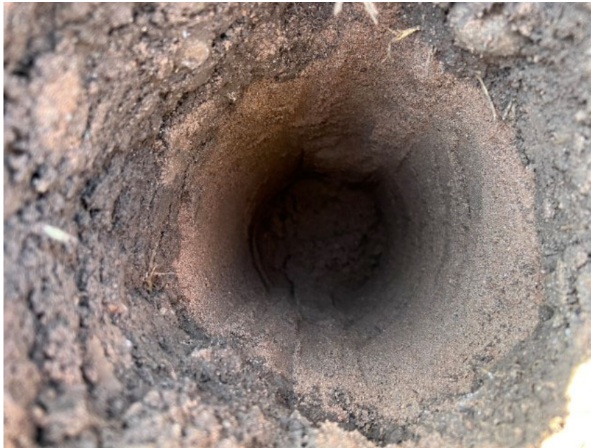
Photograph 21: Photograph shows the nature of the inert cover within the validation hole in the rear garden of Plot 237. Photograph taken 13 th September 2023.
