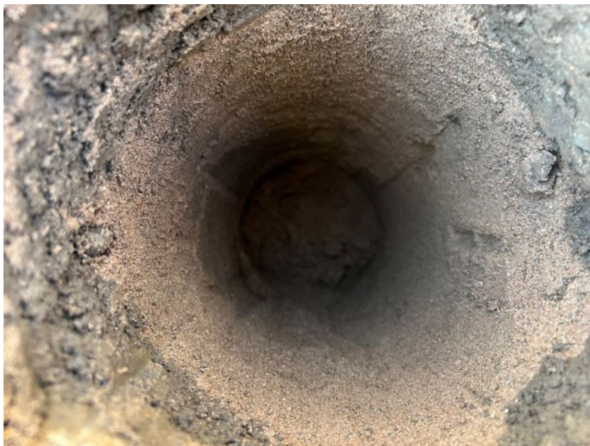
Photograph 6: Photograph shows the nature of the inert cover within the validation hole in the rear garden of Plot 232. Photograph taken 13 th September 2023.
