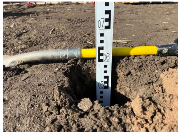
Photographs 10 & 11: Showing the depth of the inert cover and location of the validation hole within the rear garden of Plot 234 and the depth of inert cover achieved. Photographs taken 13 th September 2023.
