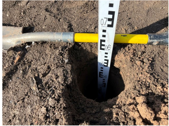
Photographs 7 & 8: Showing the depth of the inert cover and location of the validation hole within the rear garden of Plot 233 and the depth of inert cover achieved. Photographs taken 13 th September 2023.
