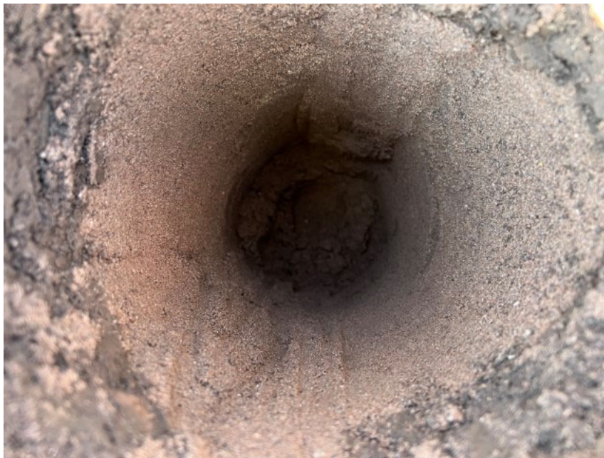
Photograph 9: Photograph shows the nature of the inert cover within the validation hole in the front garden of Plot 233. Photograph taken 13 th September 2023.
