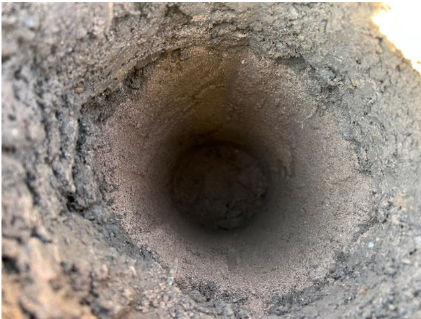
Photograph 12: Photograph shows the nature of the inert cover within the validation hole in the front garden of Plot 234. Photograph taken 13 th September 2023.
