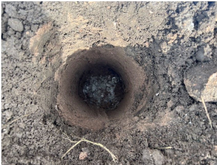
Photograph 24: Photograph shows the nature of the inert cover within the validation hole in the front garden of Plot 234. Photograph taken 20 th September 2023.
