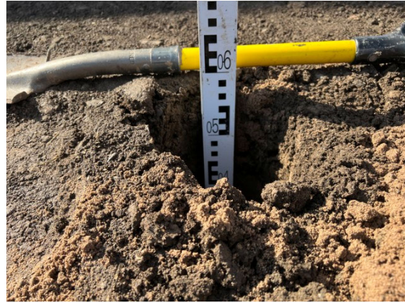
Photographs 13 & 14: Showing the depth of the inert cover and location of the validation hole within the rear garden of Plot 235 and the depth of inert cover achieved. Photographs taken 13 th September 2023.
