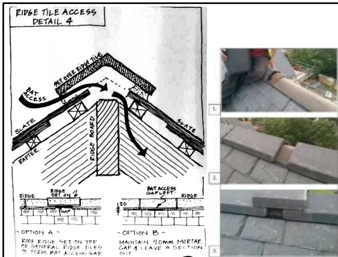
Ridge tile access creation
