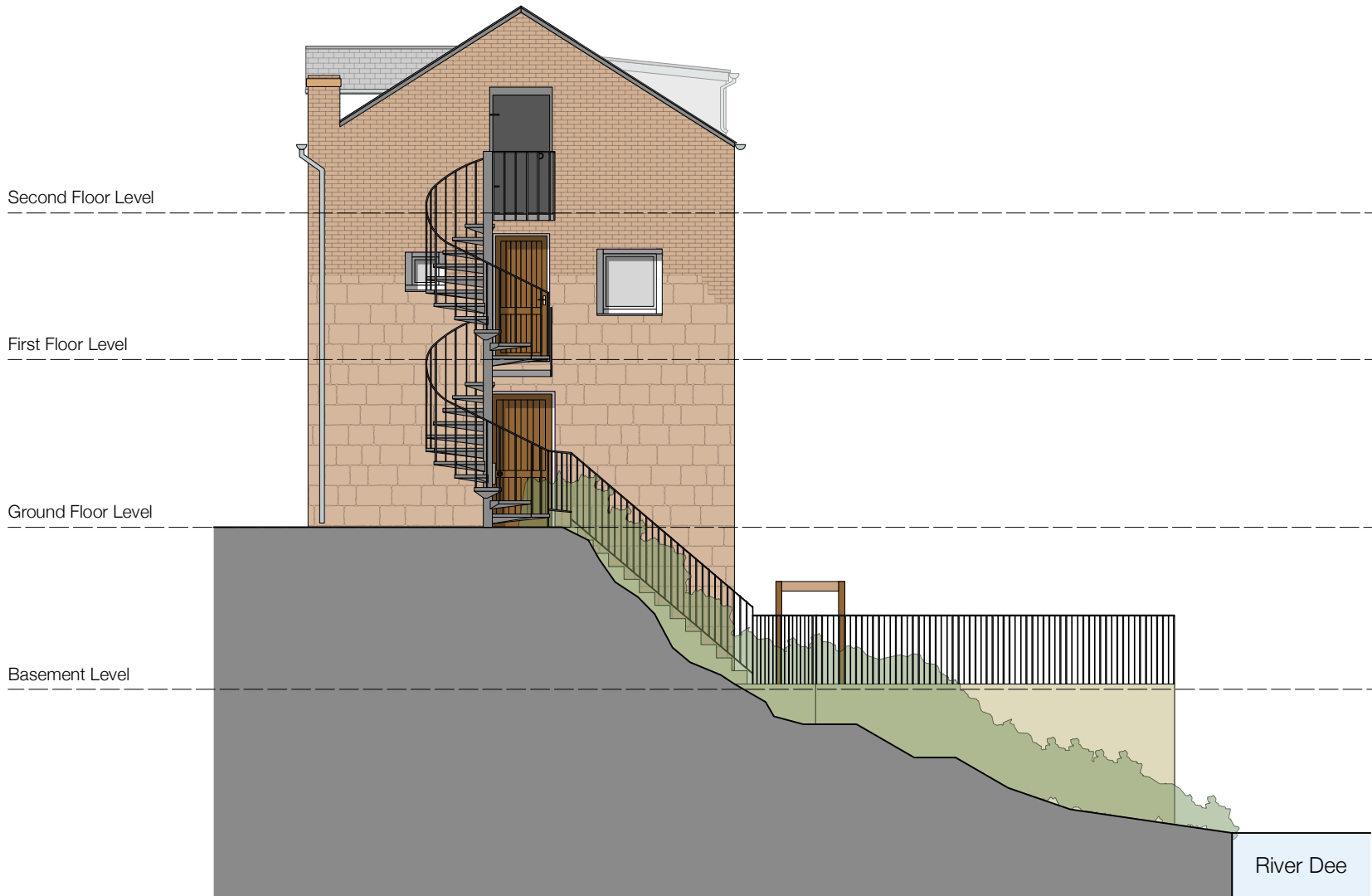
E03 Existing South Elevation
