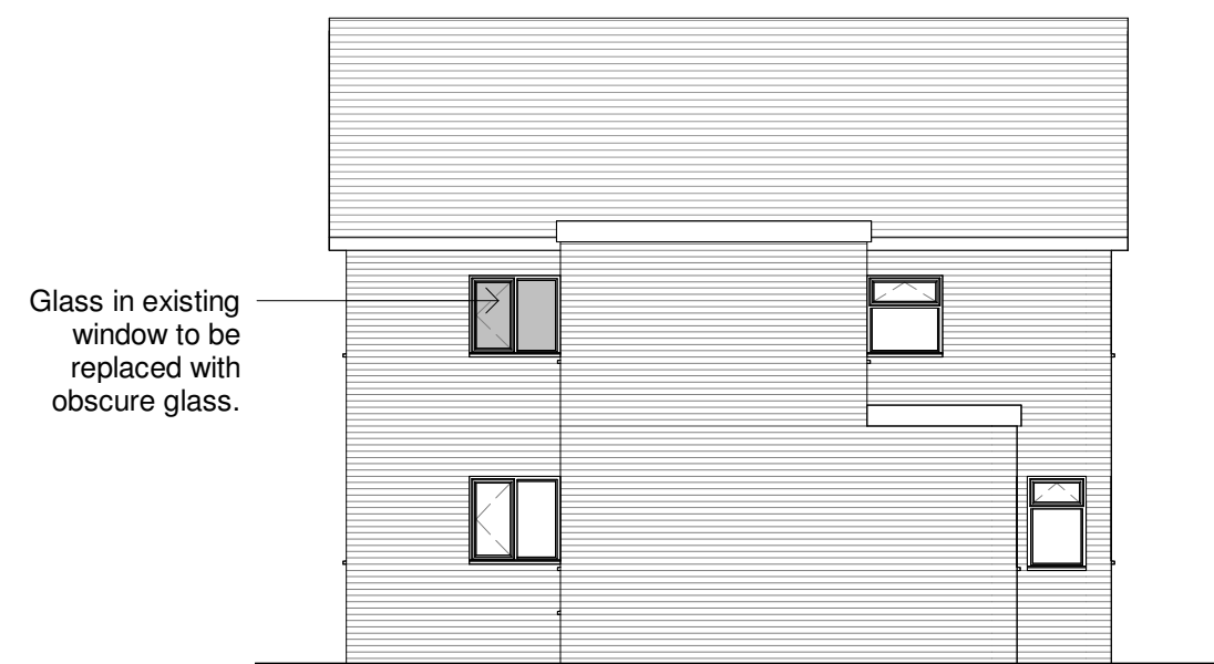
224 Holt Rd - East Elevation 1 : 100
