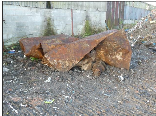
Former underground storage tank
