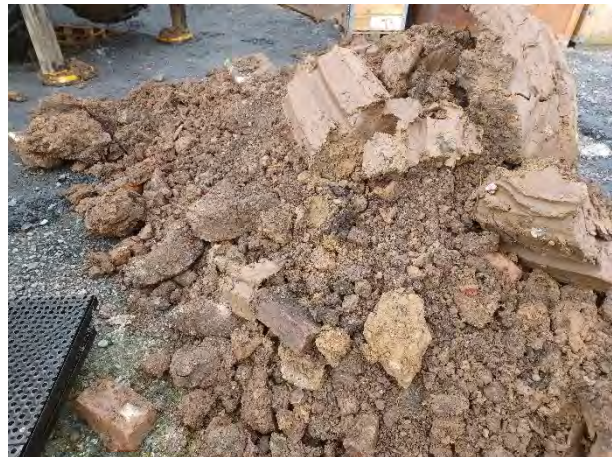
Arisings: Reworked clay (made ground) 0.5-2m with pieces of boulder clay (natural) 2-2.4m
