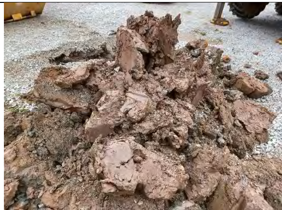
Arisings: Boulder clay 0.5-1.7m
