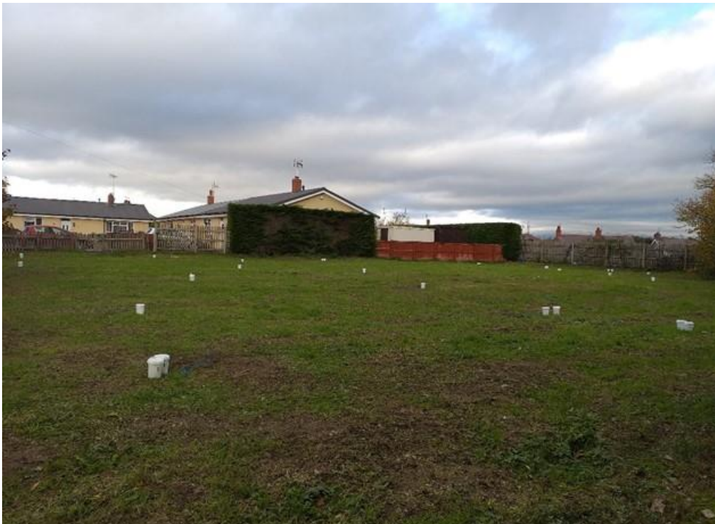
Photo 34: Spread of hand pit locations across site (soil samples taken at all locations).
