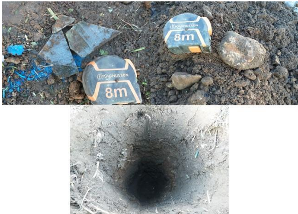
Photo 5: HP03 features of interest: Top left- reinforced glass found from 0.05 to 0.1mbgl. Top right- rare cobbles of concrete found in made ground (0.05 to 0.7mbgl). Bottom- Plastic sheeting seen in hand pit walls 0.1 to 0.25mbgl.
