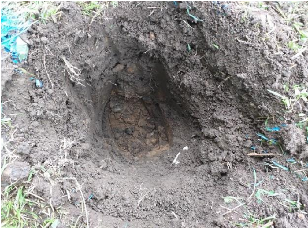
Photo 13: HP07 shallow made ground, natural material clearly visible at base of hand pit.
