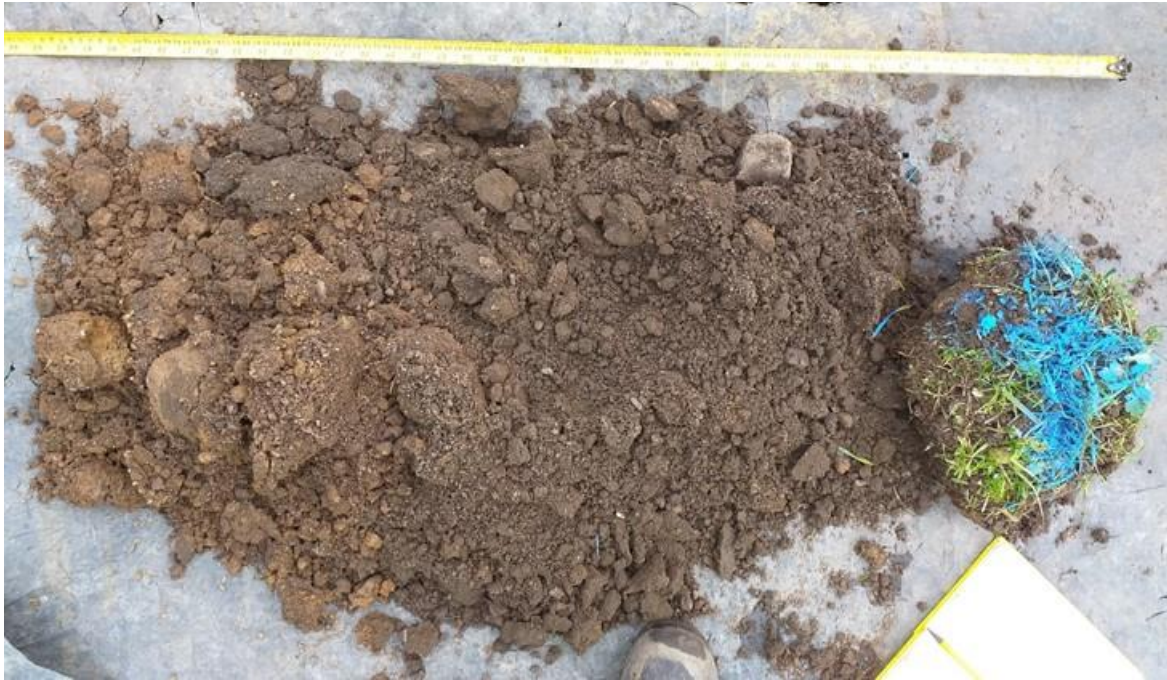
Photo 33: HP20 arisings recovered from 0 to 0.7mbgl. Depth below ground increases from right to left of image.
