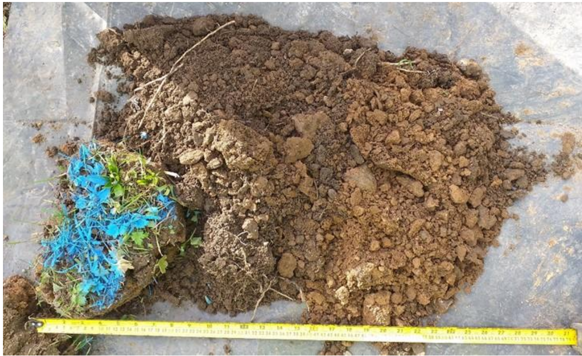
Photo 25: HP14 arisings recovered from 0 to 0.4mbgl. Depth below ground increases from left to right of image.
