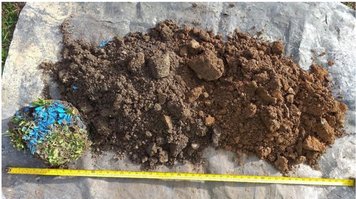
Photo 26: HP15 arisings recovered from 0 to 0.6mbgl. Depth below ground increases from left to right of image.
