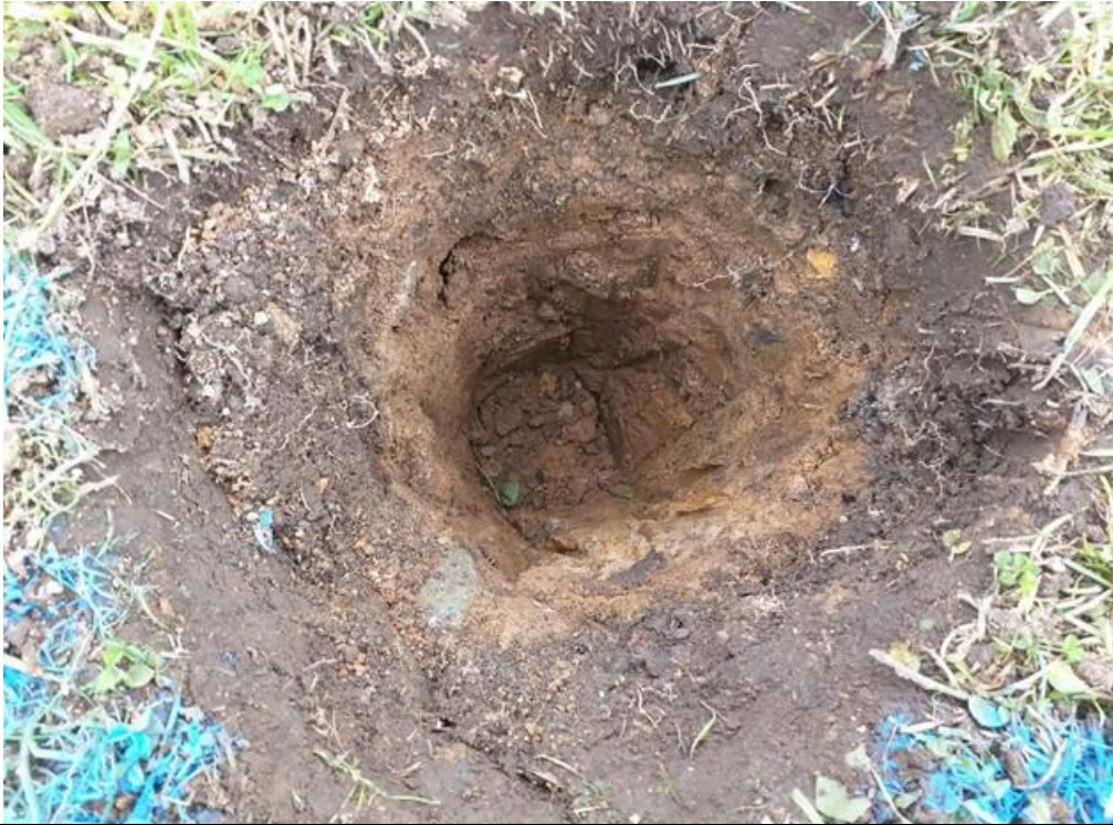
Photo 17: Shallow made ground (0.09 to 0.2mbgl) in HP09, natural material clearly visible in hand pit.
