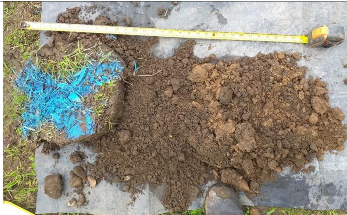
Photo 12: HP07 arisings recovered from 0 to 0.4mgb-l-shallow made ground (0.1 to 0.3mgb). Depth below ground increases from left to right of image.
