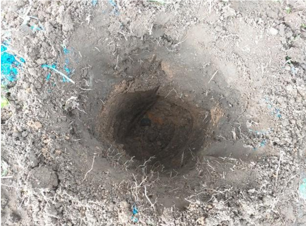
Photo 21: HP11 shallow made ground (0.05 to 0.25mbgl) so natural material is visible in hand pit.
