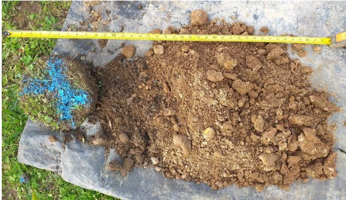
Photo 23: HP13 arisings recovered from 0 to 0.45mblg. Depth below ground increases from left to right of image.
