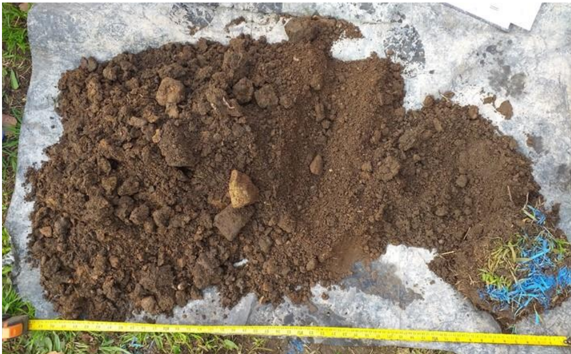
Photo 6: HP04 arisings recovered from 0 to 1.02mbgl. Depth below ground increases from right to left of image.
