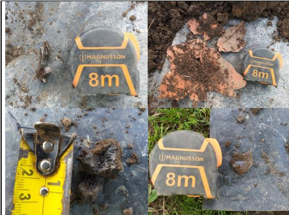
Photo 11: HP06 features of interest in made ground (0.05 to 0.55mgb): top left- plastic wrapping, top right-brittle plastic plant pot, bottom left-black combustible material, bottom right-glass fragments.
