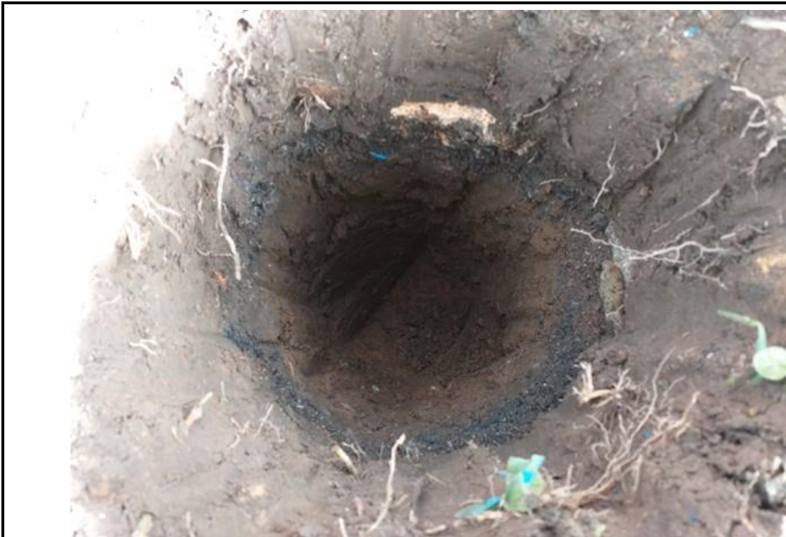
Photo 27: HP15 greyish black ashy horizon visible at 0.2 to 0.25mbgl within made ground (0.09 to 0.3mbgl). Orangish brown natural material visible below made ground (0.3 to 0.6mbgl).
