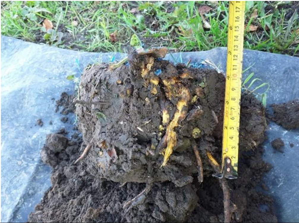
Photo 3: HP02 topsoil to 0.1mbgl containing roots.
