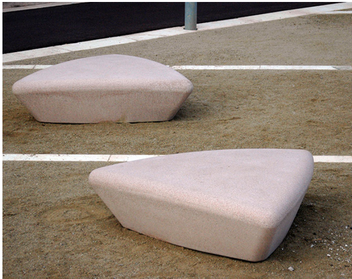
Proposed Triangular Seating (F4) Product: Escofet - Extasi (or similar approved) Dimensions: 1650 x 1650 x 460 mm Material: Cast Stone
