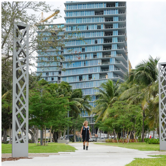
Proposed Gateway Lighting Pillar (L5) Product: Open Pillars (Streetlife or similar approved) Dimensions: 4500 mm Height Colour: Anthracite Grey Finish: Powder Coating
