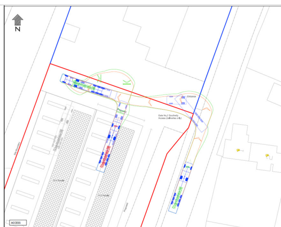
Proposed Access arrangements for HGV to extension
