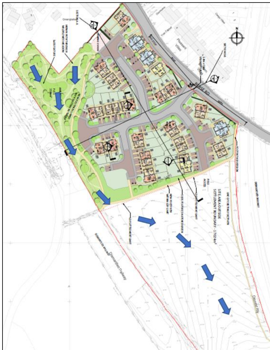
Figure 7: Development Layout with Flood Water Flow Path
