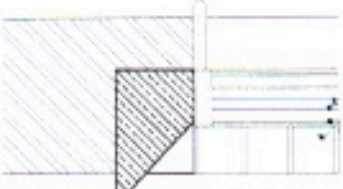
PROPOSED CILL SECTION (NTS)
