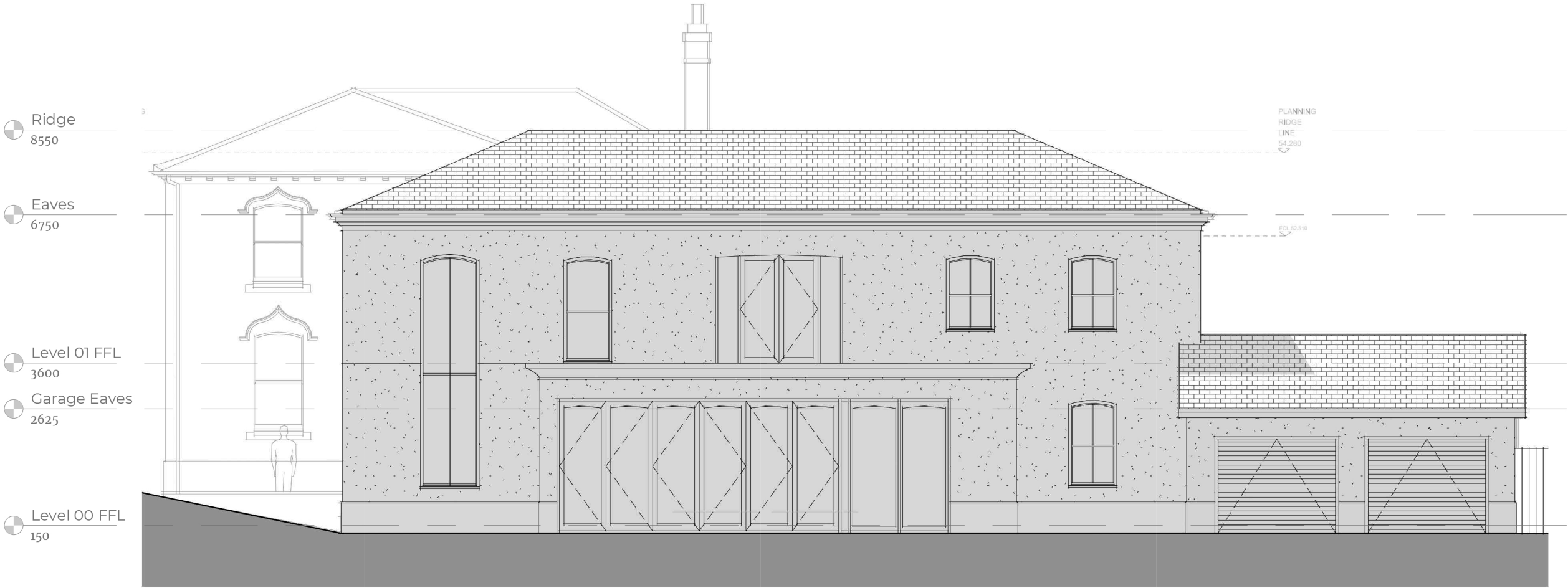
East Facing Elevation 1:100
