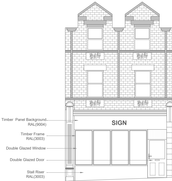
Pre-Existing Front Elevation
