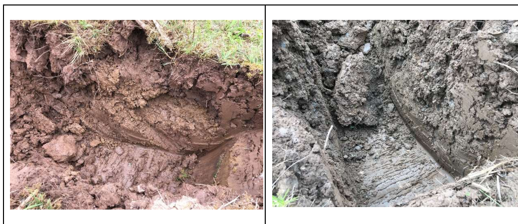
Figure 7: Typical Trial Pits made during Contaminated Ground Assessment (May 2022)
