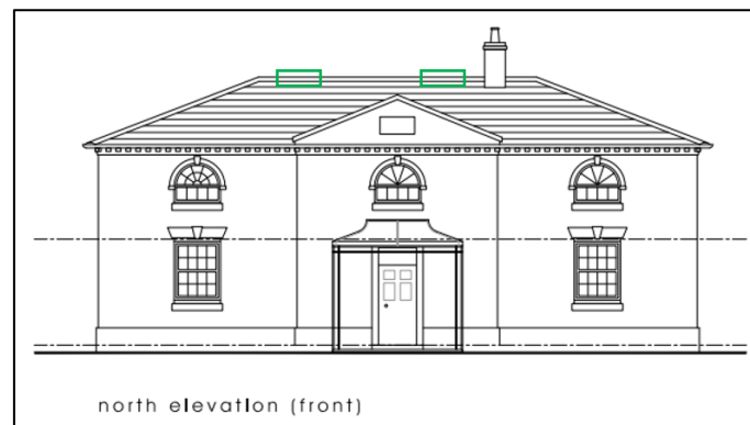
Figure 11. Creation of access and roosting opportunities under lifted ridge tiles in new roof
