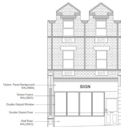
Pre-Existing Front Elevation
