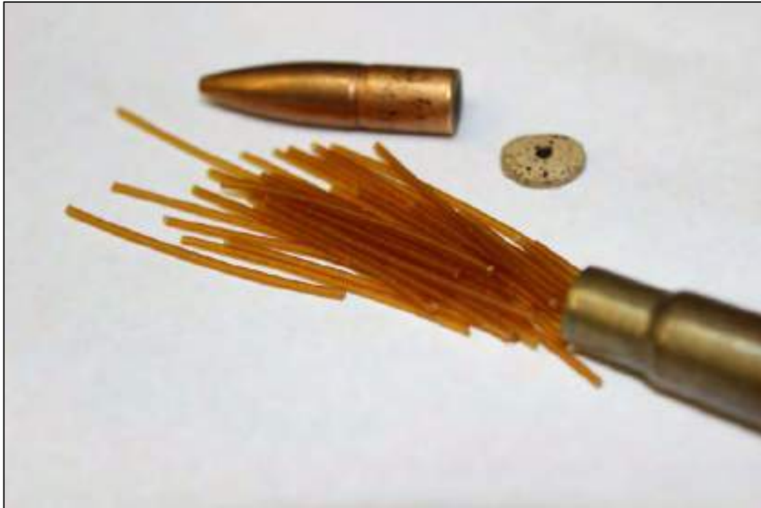
Plate 3 Cordite filaments in a .303 British Rifle cartridge
