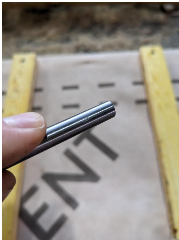
the 8 mm drill bit used to test the potential for bat access
