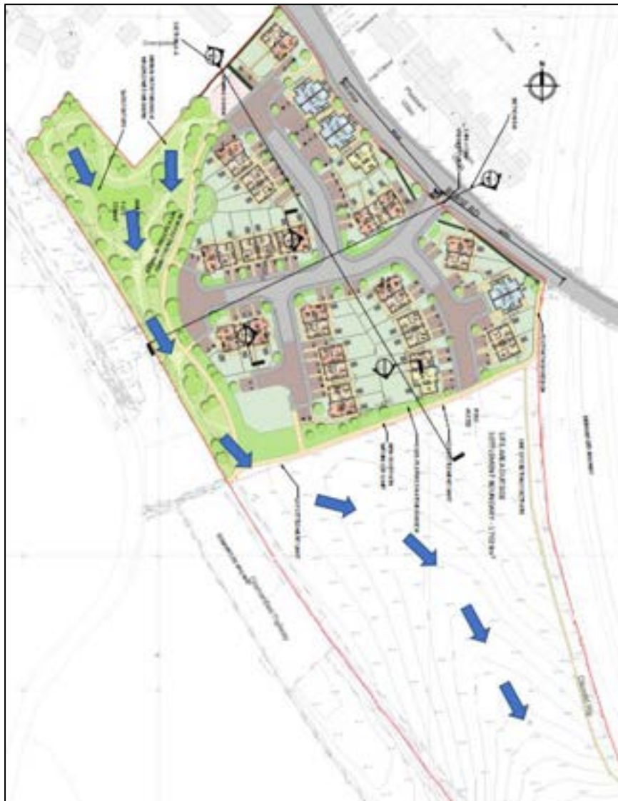
Figure 7: Development Layout with Flood Water Flow Path
