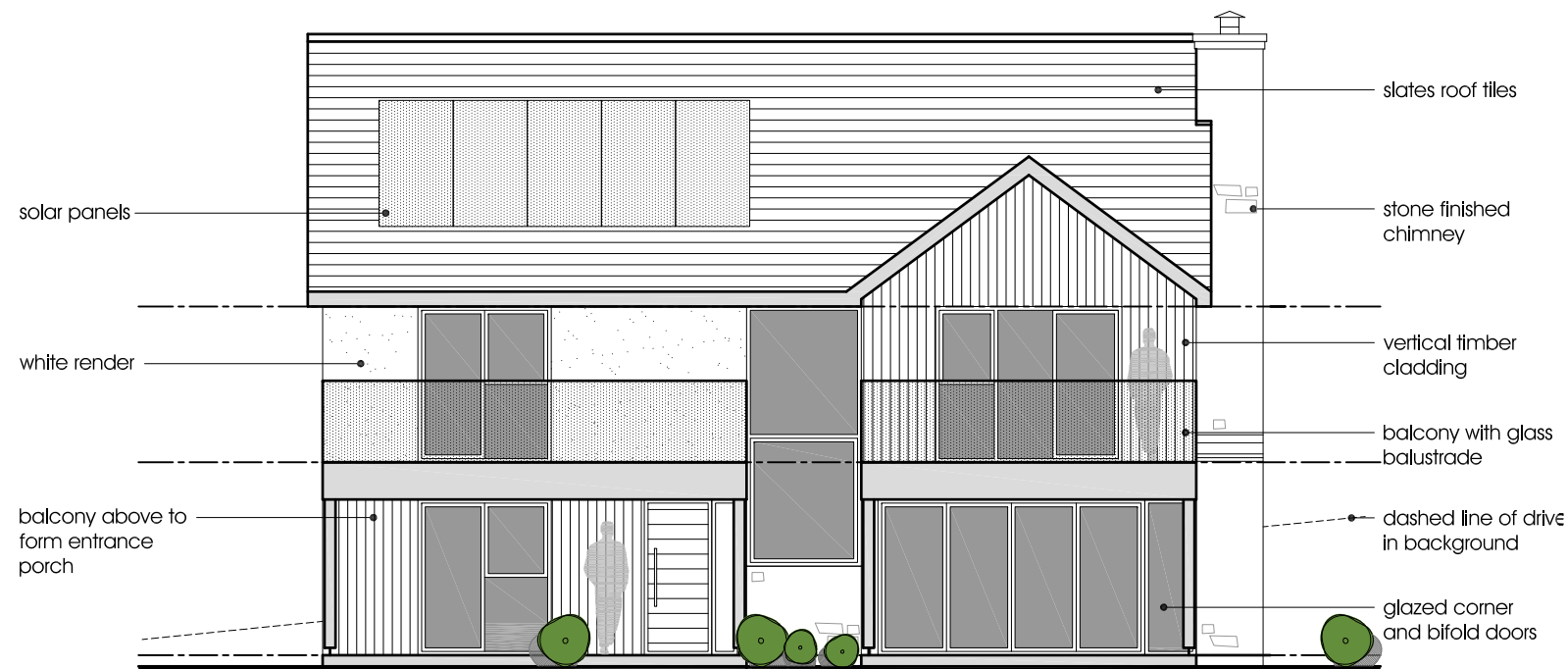
South Elevation (Rear)
